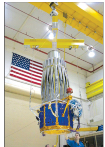
Photo 2: TacSat-4 module assembly with integrated ACT loop heat pipe system
