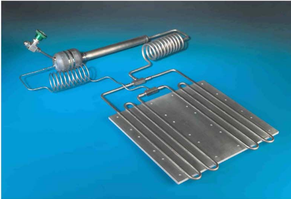
FIGURE 3. Photograph of the fully assembled titanium/water LHP.
