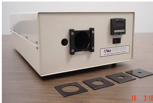
Water HPBCs installed in an enclosure with controls, temperature sensor wells, and selectable aperture plates.
