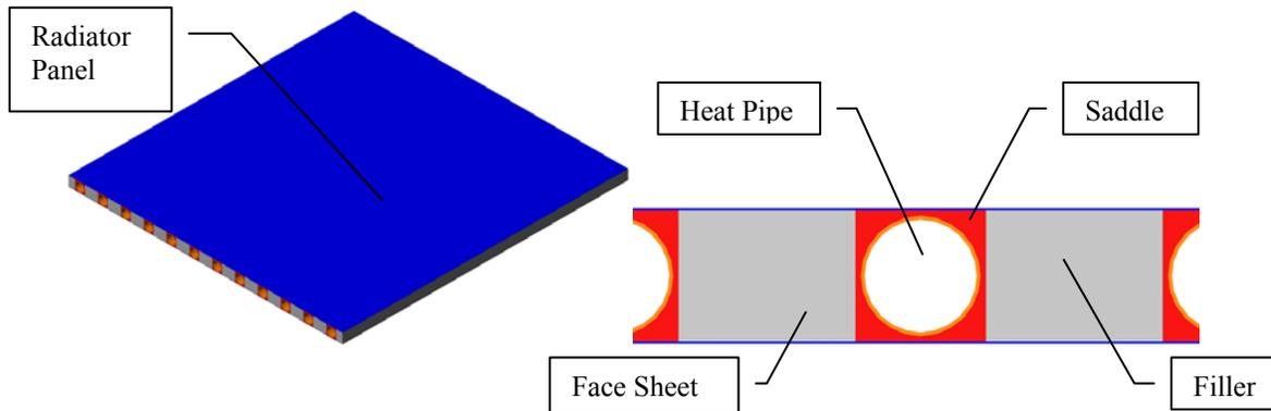
FIGURE 1. Conceptual Sketch of a Heat Pipe Radiator Panel.
