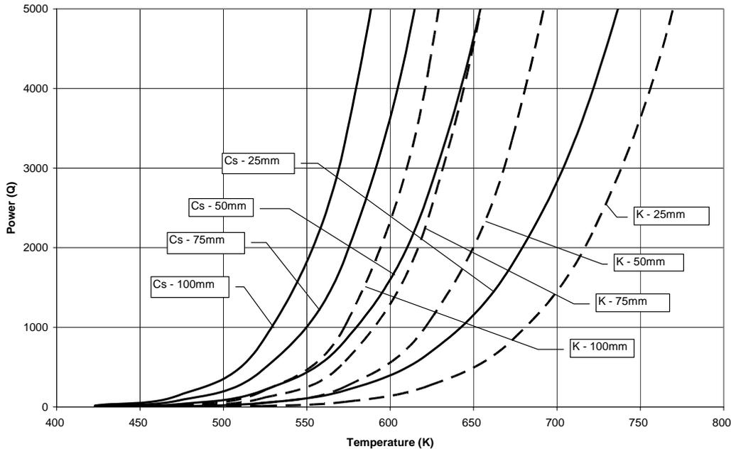
**FIGURE 5.** Sonic Limit as a Function of Heat Pipe Diameter – Cesium and Potassium
