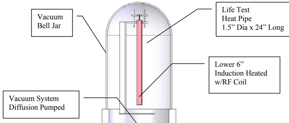
**FIGURE 8.** Heat Pipe Processing and Testing Setup.
