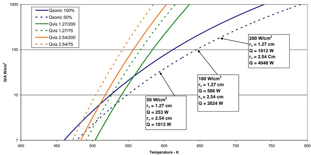
FIGURE 3. Sonic and Viscous Q/A vs. Temperature – Cesium Working Fluid.
