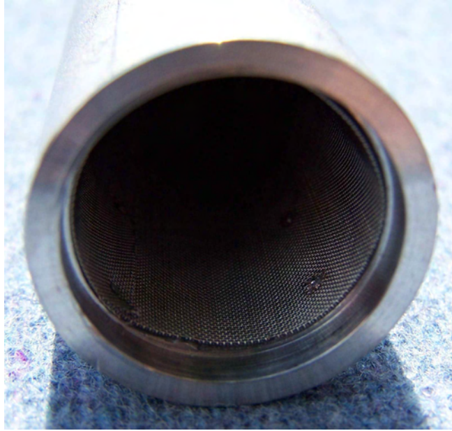
Figure 9. A screened 304 stainless steel life test heat pipe for the Therminol VP-1 life tests is pictured. The 3/4 inch Schedule 40 life test pipes are 30.5 cm long.
