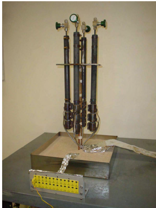
Figure 15. Cesium Copper/Nickel and Monel life test heat pipes.
