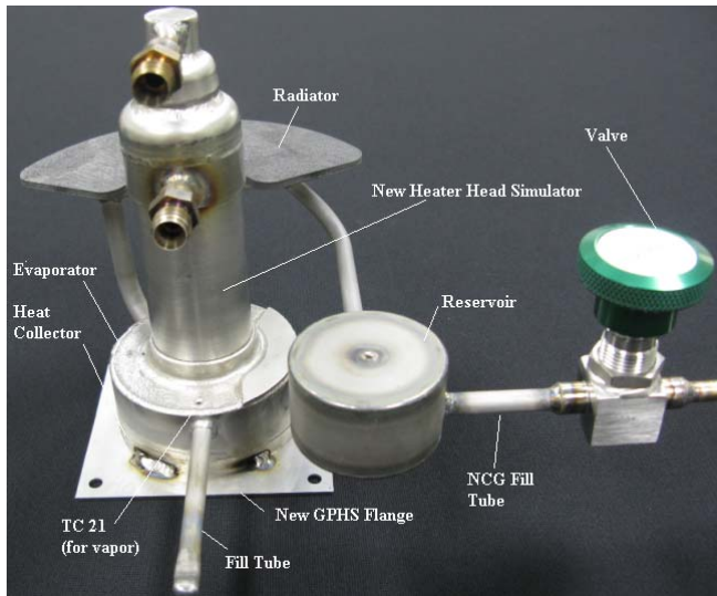
Figure 7. Prototype VCHP.
