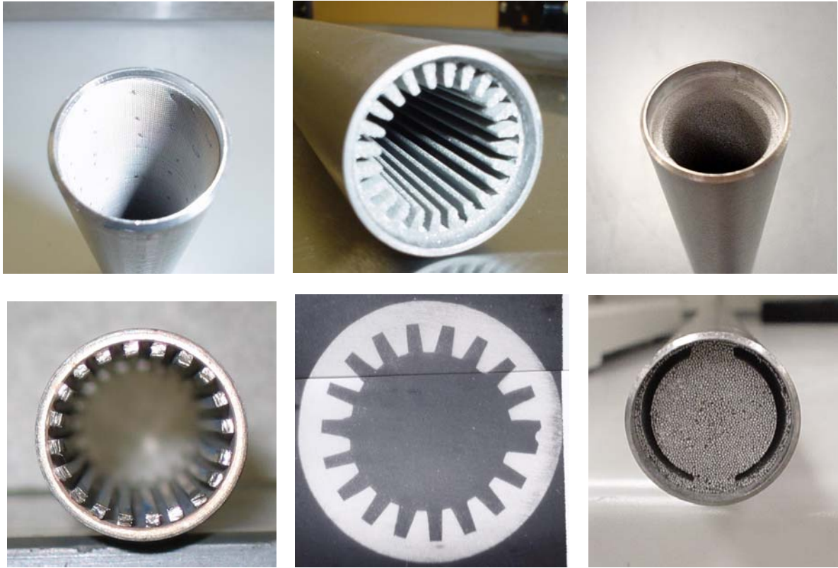
Figure 3: Survey of wick structures produced in titanium and monel which shows equivalence to structures currently produced in copper.
