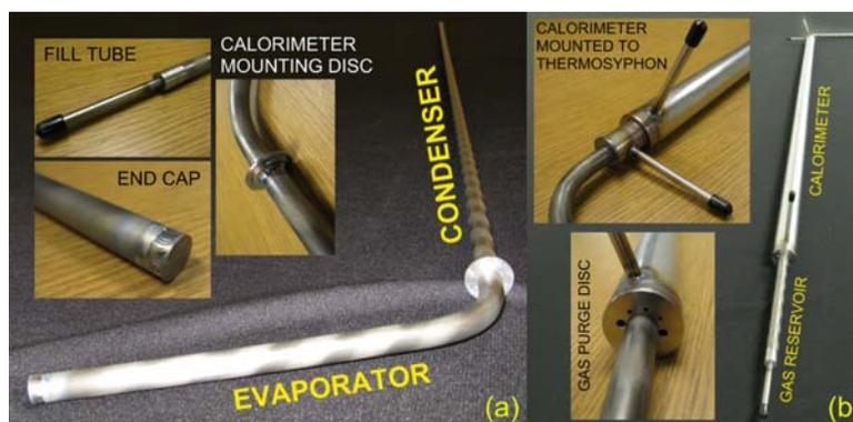
FIGURE 1. (a) Experimental VCHP and (b) Calorimeter Mounted to VCHP
