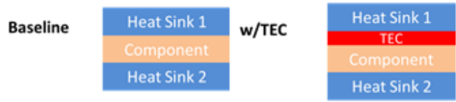
Figure 11: Dual heat sink scenario in which a TEC is placed on one side of a component to increase heat dissipation to one of two heat sinks, and its baseline comparison in which both heat sinks are unassisted.
