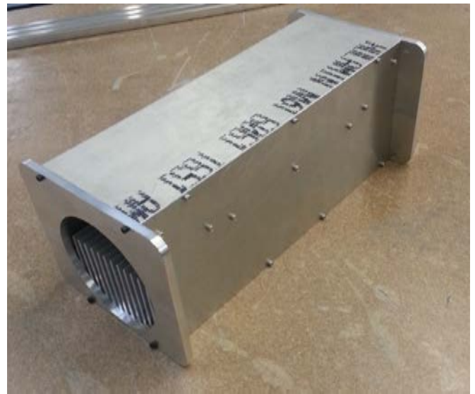
Figure 10. Heat Sink in Duct.
