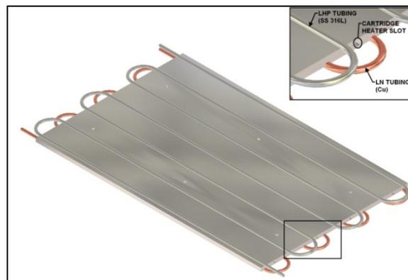
*Figure 8. LHP Condenser Design for the Test Unit*
