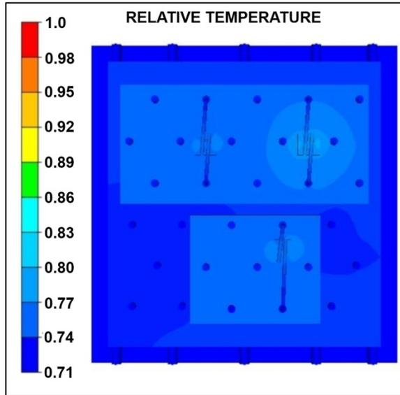
*Figure 18. FEA Model Results for Direct-Cooling Heat Pipes, Embedded Heat Pipes, and Insulation*
