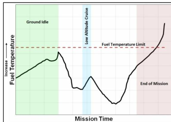
*Figure 1. Fuel Temperature during a Generic Mission<sup>3</sup>*
