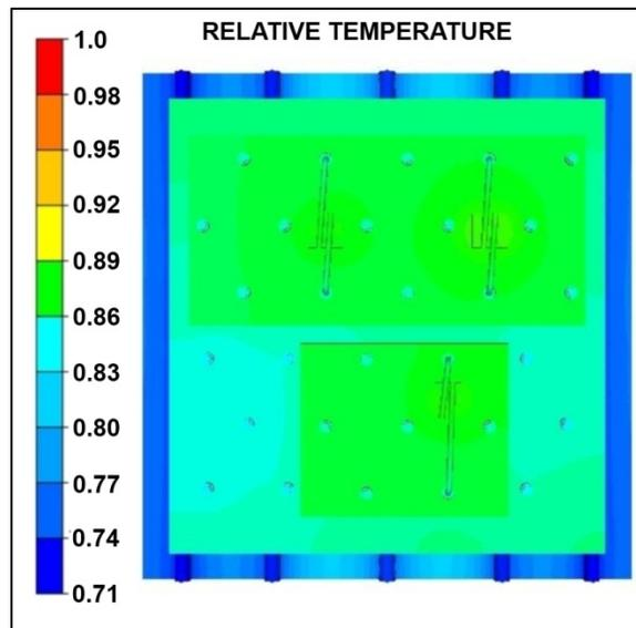
*Figure 14. FEA Model Results for Direct-Cooling Heat Pipes*
