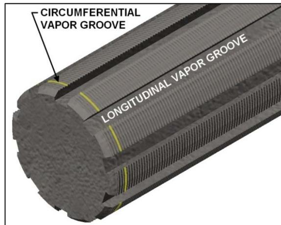
**Figure 3. Example of the Grooved Outer Surface of a LHP Wick**
