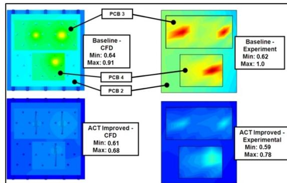
**Figure 20. Thermal Profile Comparison of the Experimental Data and Numerical Results**
