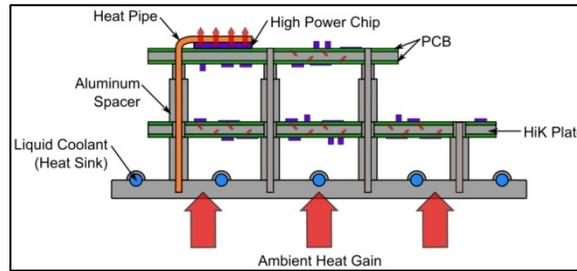
*Figure 13. Diagram of Direct-Cooling Heat Pipe Layout*
