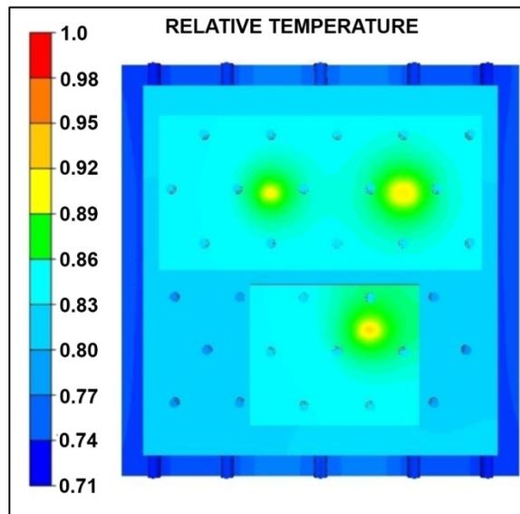
**Figure 16. FEA Model Results for Embedded Heat Pipe Plates**
