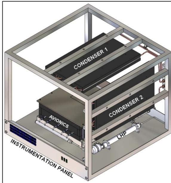
*Figure 9. LHP Design Shown Mounted in the Test Unit*
