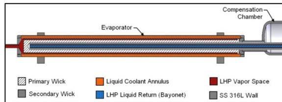
*Figure 7. LHP Evaporator Geometry for Avionics Fuel Pre-cooler*
