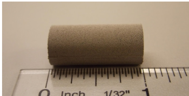
Figure 9. Sintered nickel powder (-100 US sieve size, OD = 0.5", length = 1").
