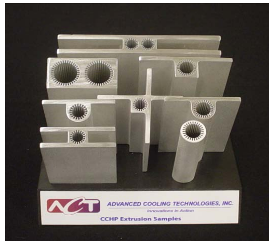
Figure 1. Grooved aluminum extrusions for ammonia heat pipes. Grooves allow long heat pipes for spacecraft applications, but only work about 0.10 inch against gravity for earth-based testing.
