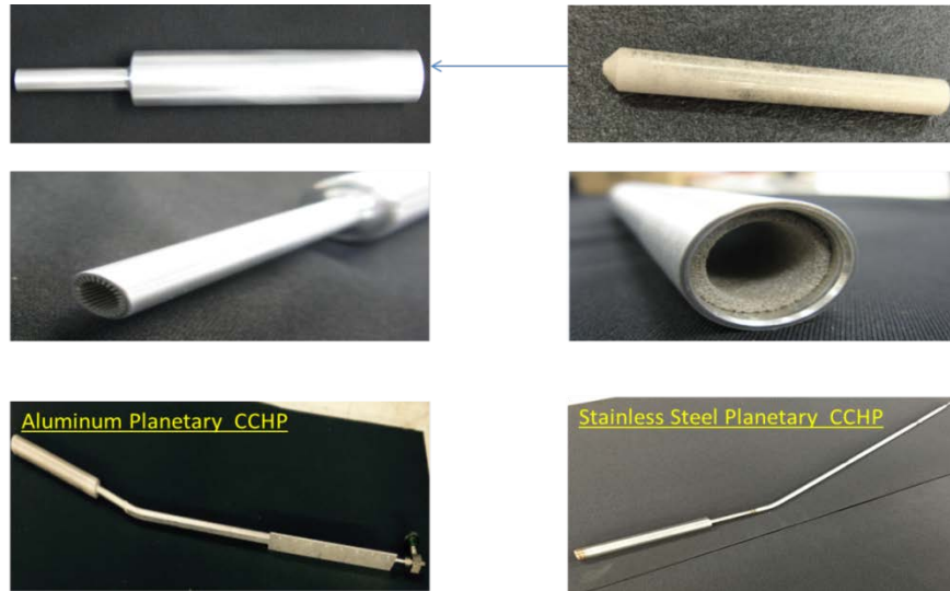
Figure 15. Planetary CCHPs assembly: The top right view shows the sintered powder metal wick with end detail design ( 45^\circ ) to interface with the axial grooves. The middle right view shows the sintered wick after insertion into the aluminum extrusion and machined to establish the wick and vapor space design parameters. The lower views show the completed pipes assembly before final bending as shown in Figures 22 and 24.
