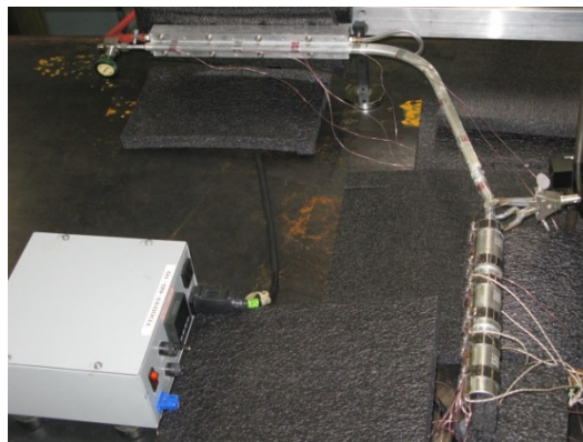
Figure 24. Thermal Link CCHP testing set up for space based orientation. The evaporator is inclined 0.1 inch to 0.3 inch to extrapolate zero-g performance.
