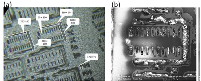
**Figure 5:** (a) Optical microscopy and (b) Scanning Electron microscopy images of different  $\mu\text{m}$ -sized grooves etched on substrate-side of GaN-on-Si filled with erythritol
