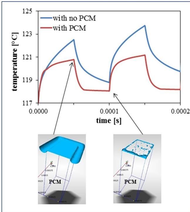
**Figure 2:** Maximum temperature rise experienced by a transistor in  $100 \mu\text{s}$  pulsed mode with 50% duty cycle. The device with the PCM (red line) experiences lower temperatures than the device with no PCM (blue line). The bottom panel shows the  $118 \text{ }^\circ\text{C}$  isotherm, which represents the PCM solid-liquid interface.
