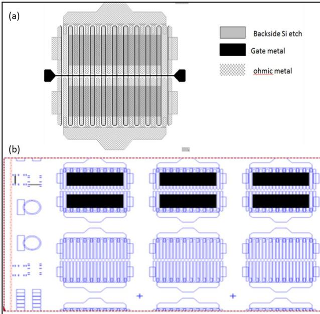
**Figure 7:** Top-view mask layout of fabricated GaN HEMTs: (a) Single transistor (b) Full mask, the horizontal black bars define the area where the silicon substrate was etched.
