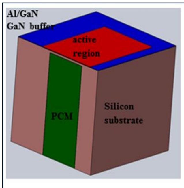
**Figure 1:** A three-dimensional model consisting of AlGaN, GaN buffer on silicon substrate with embedded PCM. The active (heat source) region is shown in red.
