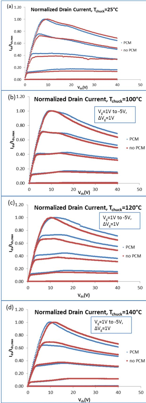
**Figure 9:** Normalized values of drain current ( $I_{ds}/I_{ds,max}$ ) as a function of drain-to-source voltage in a transistor with PCM cooling solution (red) and in a conventional transistor (blue).
