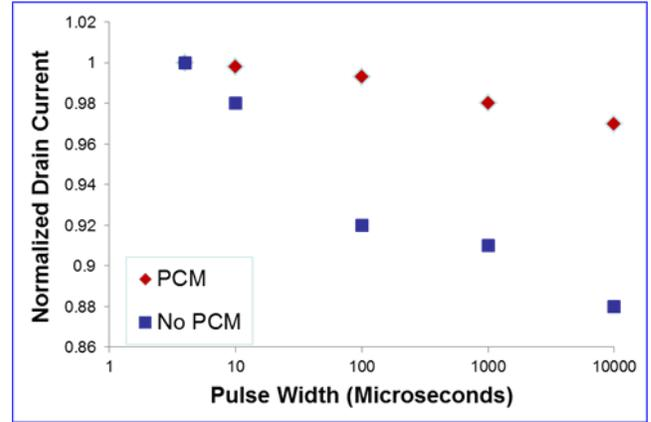
**Figure 10:** Normalized drain current in the fabricated devices as a function of the pulse width. The maximum drain current in the device with PCM is much more stable with pulse width than in the standard device.
