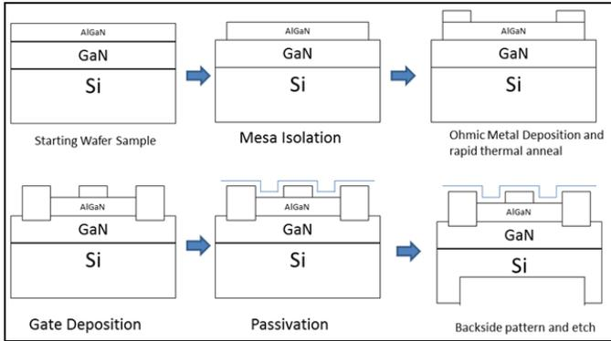
**Figure 6:** Process flow for the fabrication of PCM-enabled GaN high electron mobility transistors (HEMTs)
