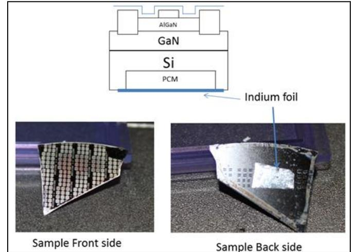
**Figure 8:** (Top) Cross-sectional image of fully fabricated AlGaN/GaN HEMT with integrated PCM, (bottom-left) Top-view image of a fabricated chip, (bottom-right) Bottom-view image of the fabricated chip showing the In foil encapsulation.
