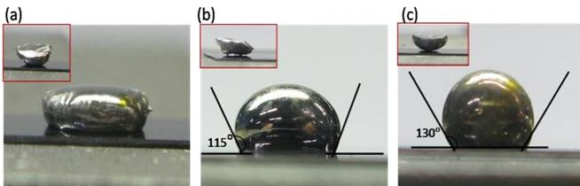
**Figure 3:** Wetting angle studies of In and  $\text{Sn}_{48}\text{In}_{62}$  on silicon wafer: (a) In melt in air (b) In melt under nitrogen (c)  $\text{Sn}_{48}\text{In}_{62}$  under nitrogen. Inset shows the solid bead before melting.
