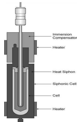
**FIGURE 6.** Cross-sectional view of the Isothermal Tower with integral copper fixed-point cell.
