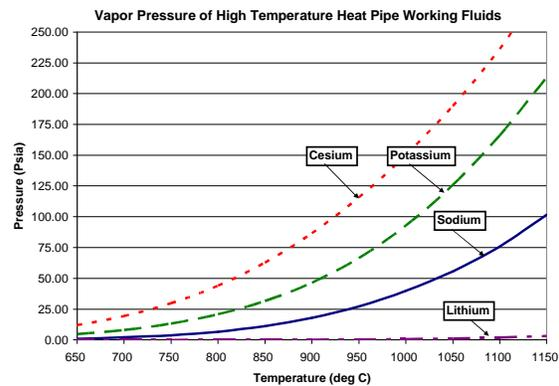
**FIGURE 3.** Vapor pressure curves for typical high temperature heat pipe working fluids.
