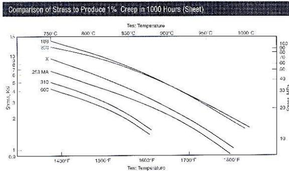
**FIGURE 4.** Stress to produce 1% creep in 1000 hours. Reprinted from Haynes International’s Haynes 230 Product Brochure ([www.haynesintl.com](http://www.haynesintl.com))
