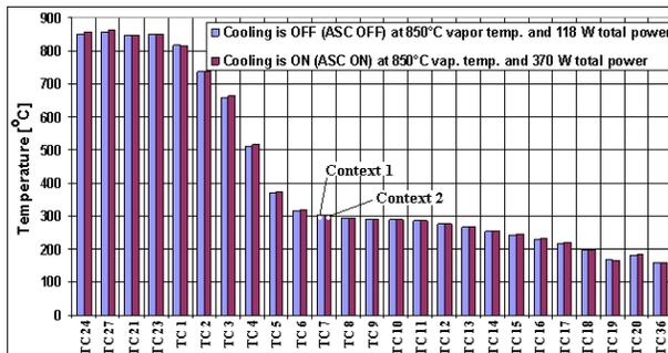
Figure 9. VCHP temperature distributions at steady state for Contexts 1 (heat loss determination) and 2 (Stirling on).
