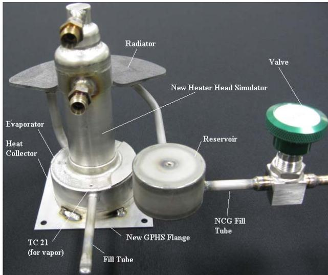
Figure 5. Prototype VCHP.
