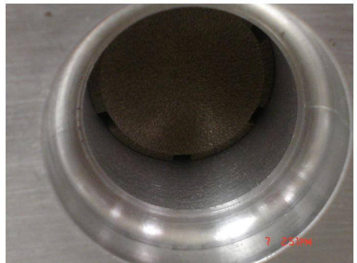
Figure 8. LHP wick inserted in the evaporator body. Note the axial grooves, which deliver the vapor to the vapor line.
