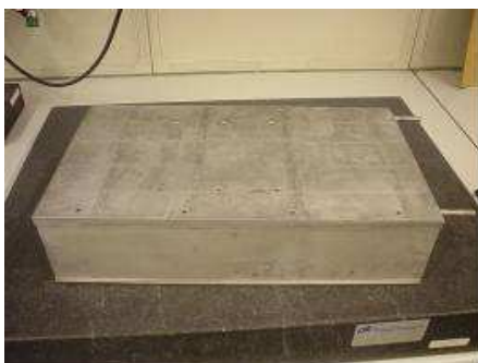
Figure 4 A heat sink incorporated with an oscillating flow heat spreader is shown. Also shown are performance predictions and test data
