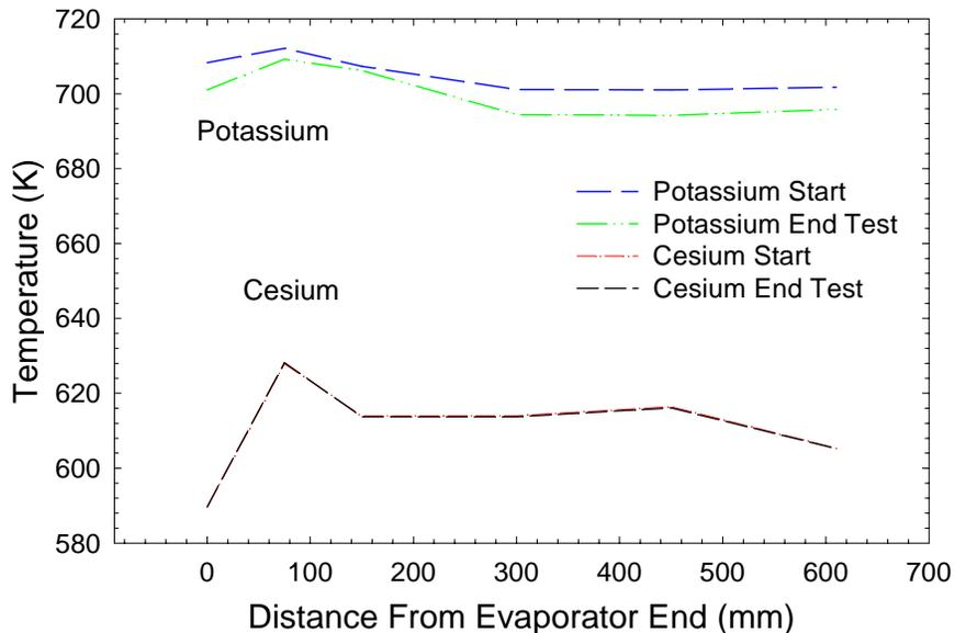
**FIGURE 9.** Life Test Heat Pipe Temperature Profiles at Start and Finish of 48 Hour Test.
