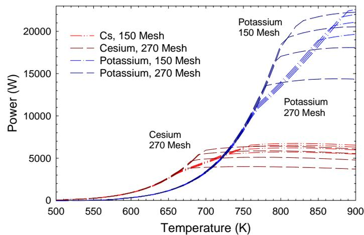
**FIGURE 7.** Cesium and Potassium Heat Pipe Limits for 50mm ID, 125mm Evaporator, 50mm Adiabatic, 2m Overall, Various Screen /Screen Artery Wicks (Each Line Within a Subgroup Represents a Different Evaporator Wick Thickness), in Space.. The Cross-Over Point for Potassium versus Cesium is Around 740 K.
