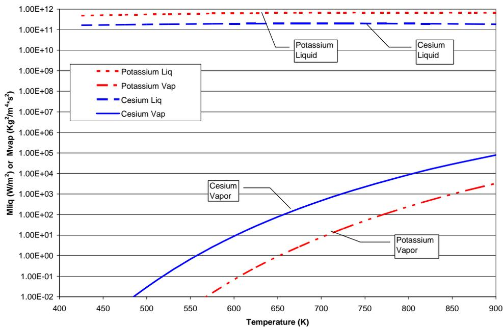
**FIGURE 2.** Liquid and Vapor Figure of Merits – Cesium and Potassium.
