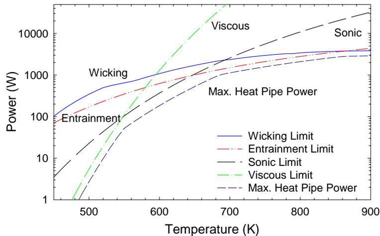
**FIGURE 6.** Heat Pipe Power Limits versus Operating Temperature. Cesium, 25mm ID, 125mm Evaporator, 50mm Adiabatic, 1m Condenser, 1.5mm Thick (-50+100) Sintered Powder Wick, in Space.
