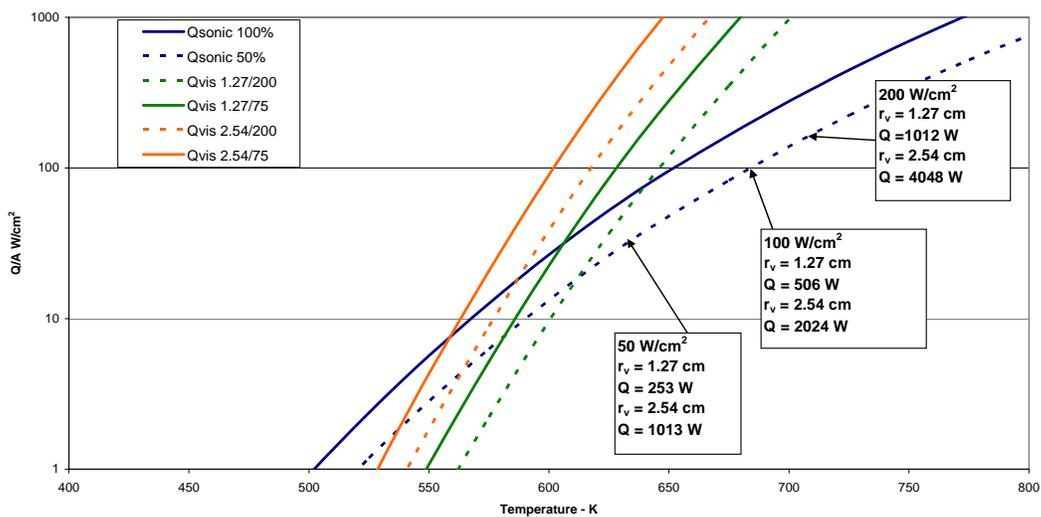
**FIGURE 4.** Sonic and Viscous Q/A vs. Temperature – Potassium Working Fluid.
