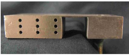
Fig. 4 A side view of the test section is shown. Thermocouples inserted in the 9 holes are used to measure the heat flux and surface temperature of the condensing surface. A gap was also machined to prevent heat from leaking in through the vapor/liquid ports.
