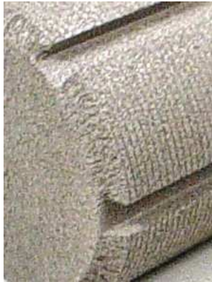
Figure 6. Detail of a LHP wick, showing the circumferential and axial grooves used to remove vapor from the heated surface.
