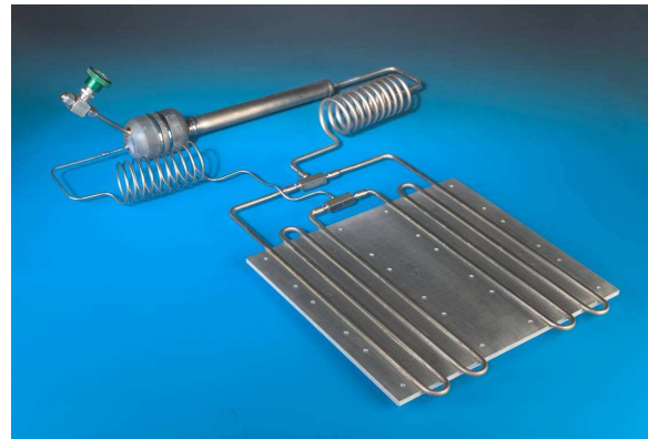
Figure 7. Titanium/water loop heat pipe that carried 590 Watts at vapor temperature of 140^{\circ}\text{C} .
