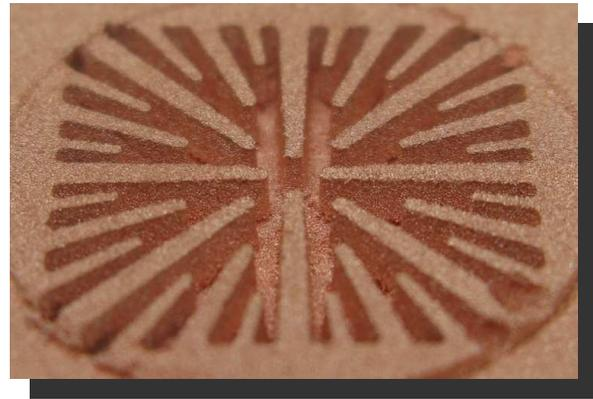
**Figure 2.** Converging Wick Structure. Thick wick fingers deliver liquid to the thin wick sections between the fingers where evaporation takes place. Vapor escapes through the spaces between the fingers [3].
