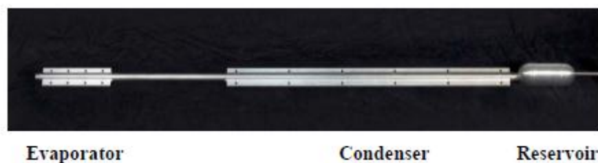
Figure 4. Standard VCHPs have the reservoir located next to the condenser.
