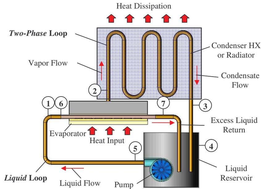
Figure 1 Schematic diagram of hybrid cooling loop.
