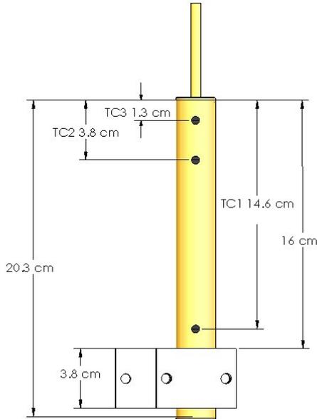
**Figure 8. Location of thermocouples and heater block.**
