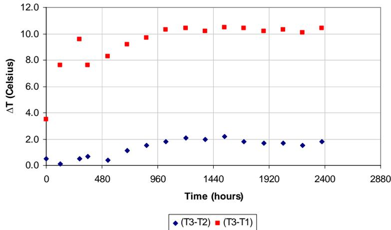
**Figure 15. Low Temperature (Non-Condensable Gas) Measurements for Monel K-500 Envelope/Monel 400 Sintered Wick/Water Heat Pipe 20, Operating at 550 K.**
