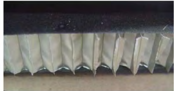
Figure 9. Close-up of Cured Sandwich Panel with High Thermal Conductivity skins.
