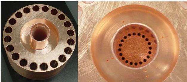
Figure 5. Photographs of the annular wick (left) and biporous slab wick with vapor vents (right) are shown.
