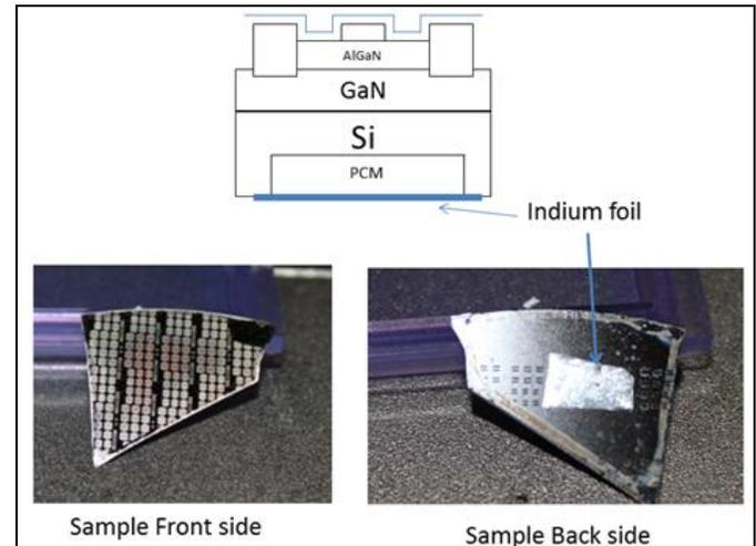
**Figure 8:** (Top) Cross-sectional image of fully fabricated AlGaN/GaN HEMT with integrated PCM, (bottom-left) Top-view image of a fabricated chip, (bottom-right) Bottom-view image of the fabricated chip showing the In foil encapsulation.
