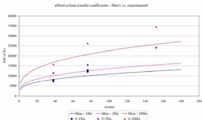
**Figure 21 Effective heat transfer coefficient at heating region – Shin's vs experimental data.**
