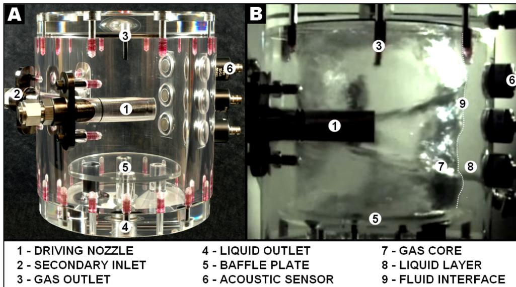
**(A) MVS designed for a microgravity two-phase system (B) during testing**
