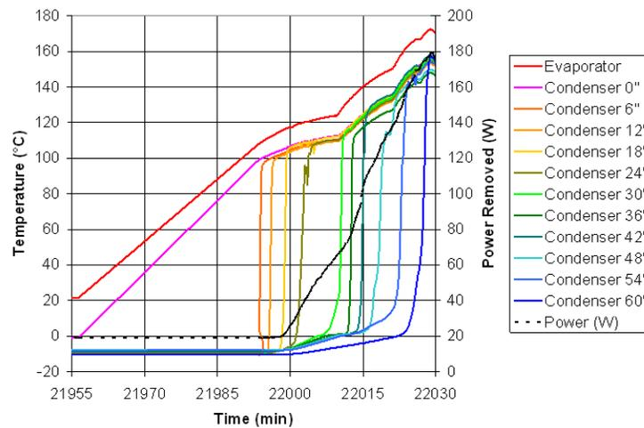
FIGURE 7. Temperature and Power Profiles for VCHP Thaw after Freezing.
