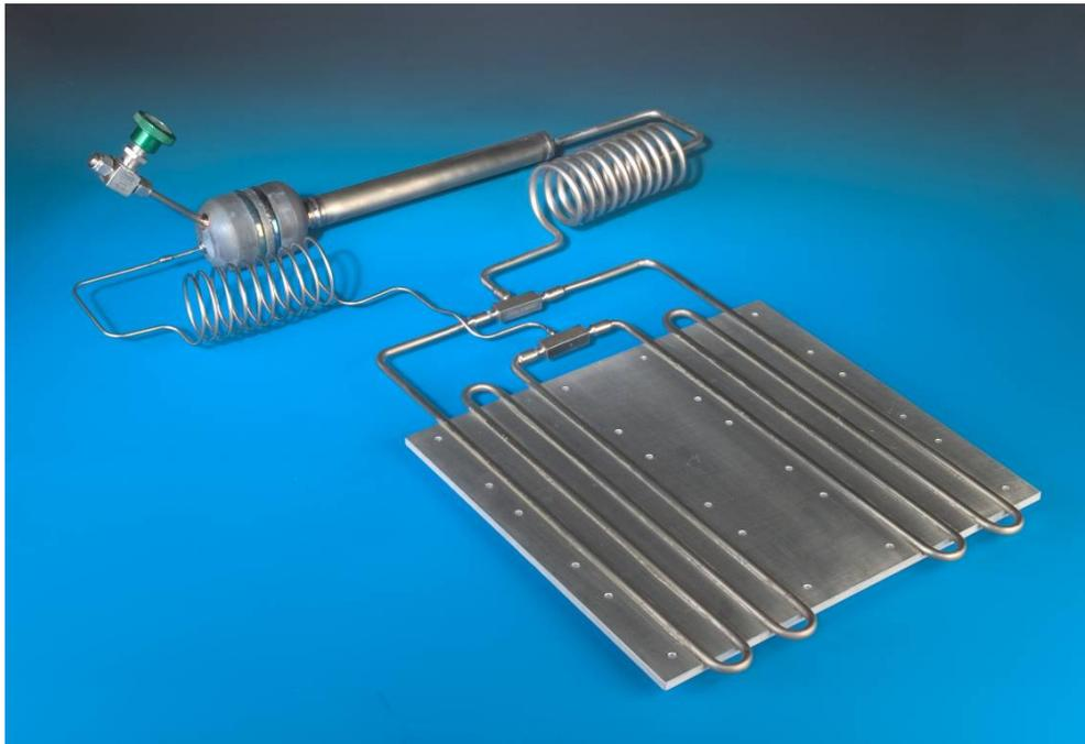
**FIGURE 3.** Photograph of the fully assembled titanium/water LHP.
