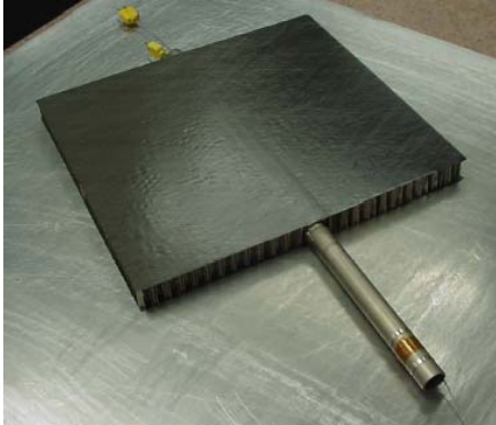
Figure 6. Test panel with embedded titanium tube
