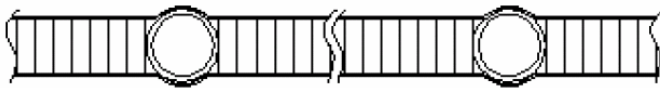
Figure 1. Configuration with heat pipes embedded in a sandwich panel with conformal face sheets.
