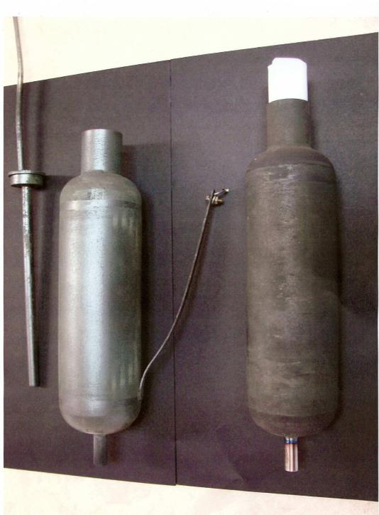
**FIGURE 7.** There is no sign of deformation or corrosion on the ultra-high temperature IFL (left side) after being operated for over 2000 hrs at 1070°C. For comparison, a second ultra-high temperature IFL is shown (right side) with zero hours of operation.
