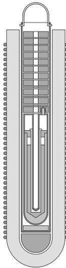
**FIGURE 1.** Schematic representation of freeze-point cell inside of an Isothermal Furnace Liner (IFL).
