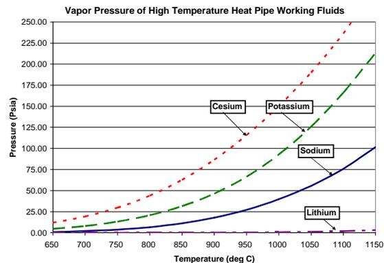
**FIGURE 3.** Vapor pressure curves for typical high temperature heat pipe working fluids.
