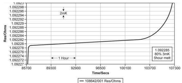
**FIGURE 2.** Typical melt plateau plot. The resistance (Ohms) of the HTPRT is directly proportional to temperature. In this chart, one milli-Kelvin is 0.000001 Ohms.
