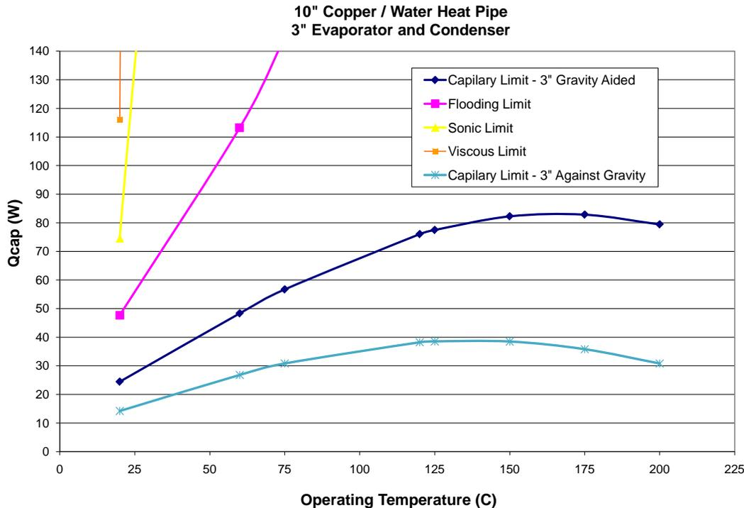
**Figure 1 Heat Pipe Performance Limits for 10" Long copper/water heat pipe. Two capillary curves show the effect of orientation.**
