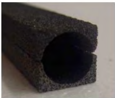
Figure 10. Close-up of Poco Foam Saddles.
