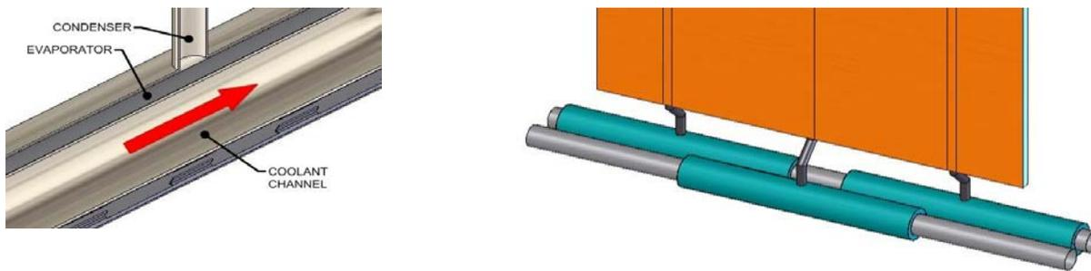
Figure 6. Annular Evaporator Concept. (a) Cross-Section. (b) Heat Pipe Evaporators Alternate between Coolant Loops.
