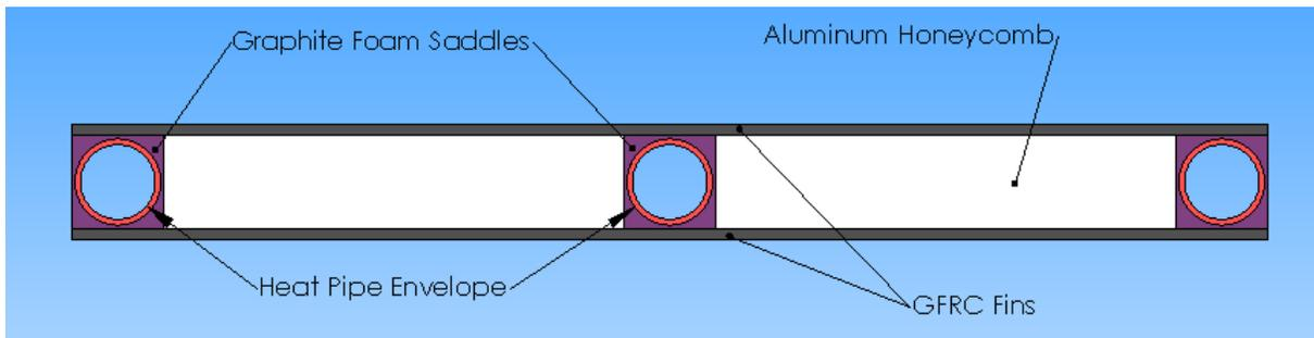
**Figure 2. Radiator Panel Cross-Section, with Titanium Heat Pipes and POCO Foam Saddles.**
