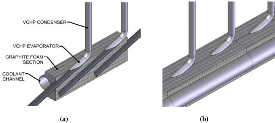
**Figure 3. (a) Graphite Saddle Concept Cross-Section, (b) Assembled Graphite Saddles.**
