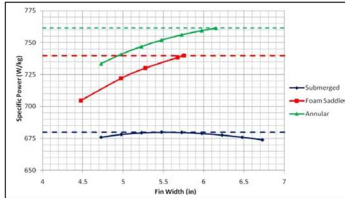
Figure 8. Comparison of Optimized Designs for Each Interface (Shackleton Crater).
