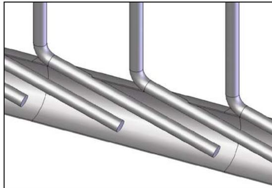
**Figure 4. Intrusive VCHP Evaporators Welded to Coolant Channel at Entry Point.**
