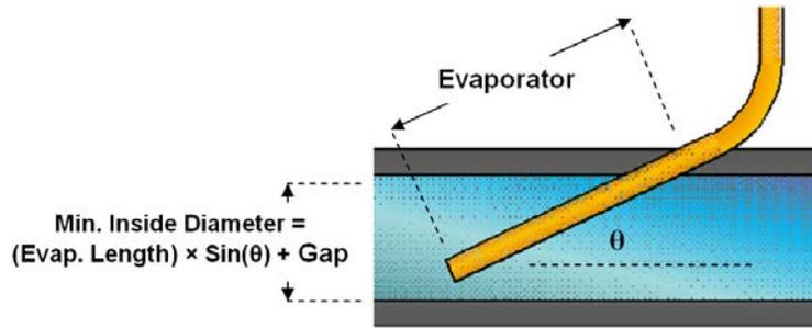
Figure 5. Coolant Channel Diameter Relationship with Evaporator Length and Angle.
