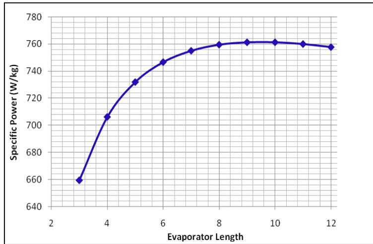
**Figure 7. Highest Possible Specific Power for a Given Evaporator Length, Annular Evaporator.**
