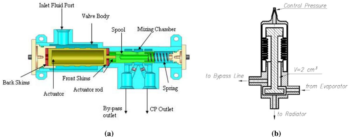
**Figure 4. Thermal Control Valve Configurations. (a) PDT valve for the Mars Science Laboratory has an actuator that does not depend on the working fluid pressure (Birur et al., 2008). (b) TCV design used by Goncharov et al. (2001, 2005) is dependent on the working fluid pressure to move the valve.**
