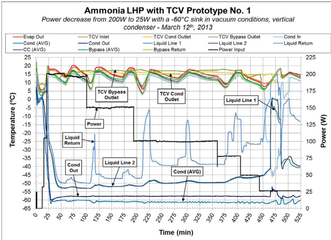
Figure 9. Ammonia LHP with TCV operating with a vertical condenser in the thermal vacuum chamber, -60°C constant sink conditions with a power input decrease from 200W to 0W.
