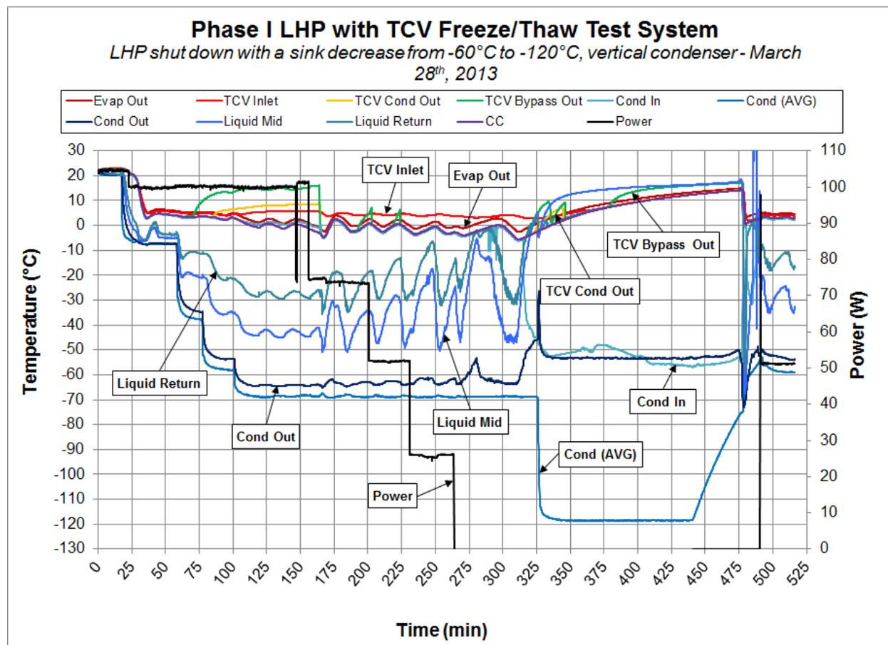
Figure 13. Ammonia LHP with TCV operation at -120°C sink during shut down with a restart of 50W.
