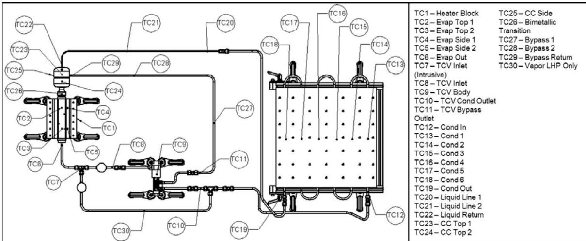
Figure 15. Propylene LHP with TCV Thermocouple map.
