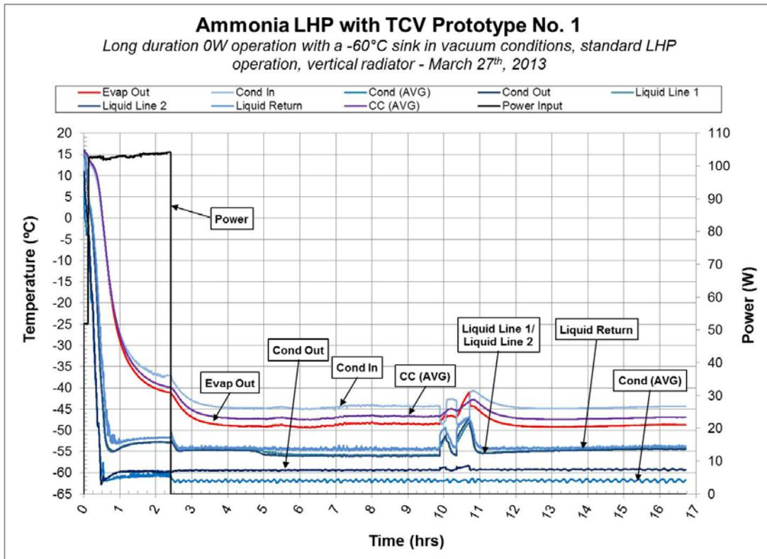
Figure 11. Ammonia standard LHP (flow is bypassed around the TCV) operating with a vertical condenser in the thermal vacuum chamber, -60°C constant sink conditions with long duration 0W power input.
