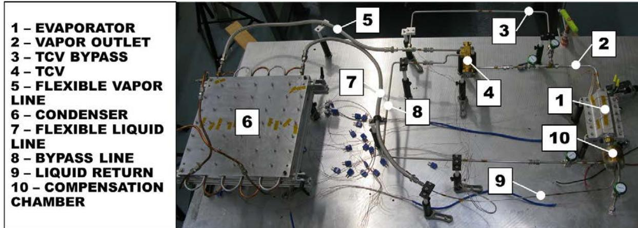
Figure 14. Propylene LHP with TCV assembly.
