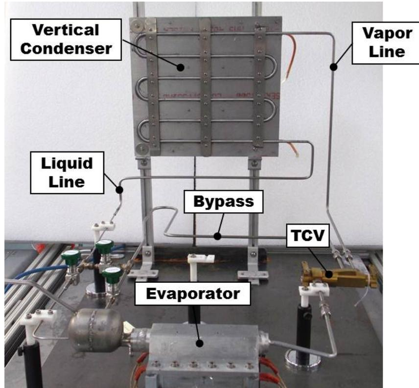
**Figure 12. Ammonia LHP with TCV freeze and thaw test assembly.**
