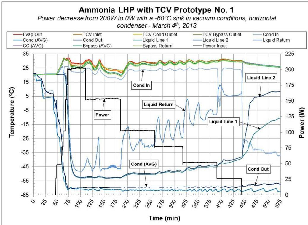
Figure 7. Ammonia LHP with TCV operating with a horizontal condenser in the thermal vacuum chamber,  $-60^{\circ}\text{C}$  constant sink conditions with a power input decrease from 200W to 0W.
