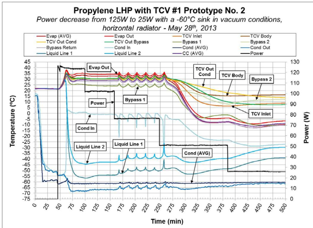
Figure 17. Propylene LHP with TCV power decrease from 125W to 25W with a  $-60^{\circ}\text{C}$  sink in vacuum conditions with a horizontal condenser.
