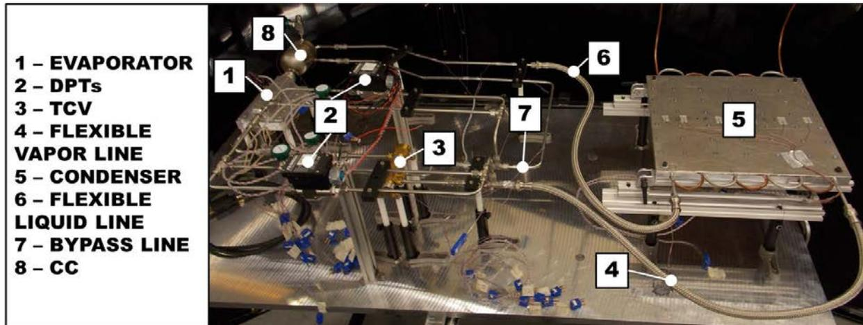
Figure 5. Ammonia LHP with TCV design.
