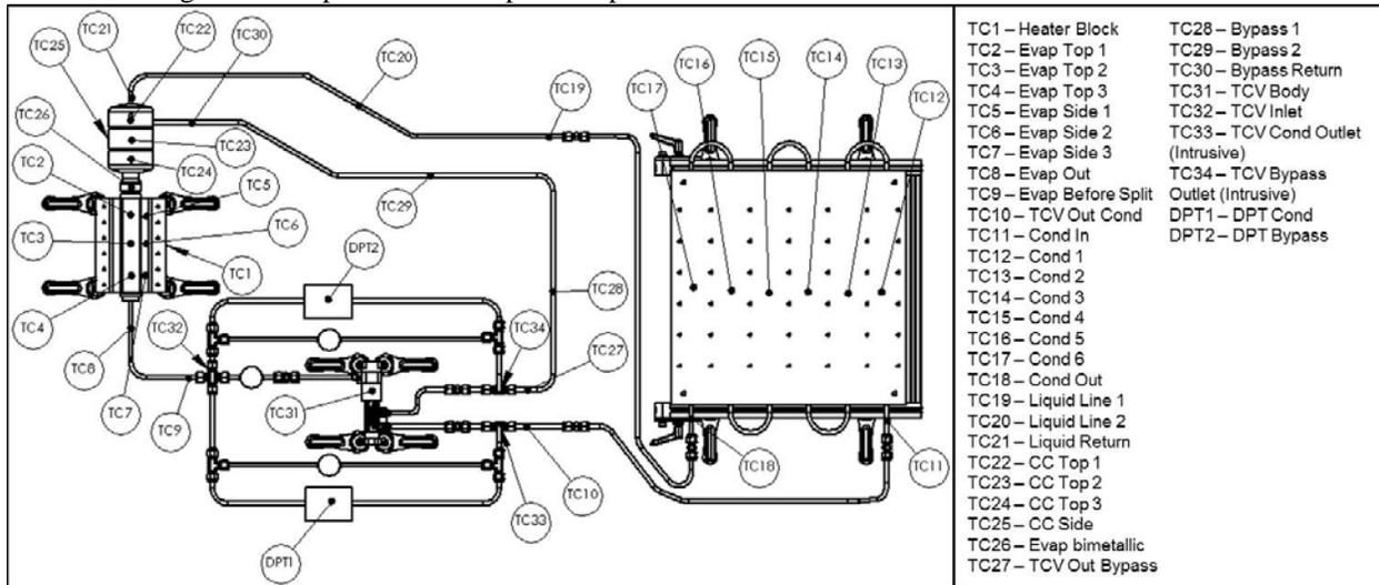
**Figure 6. Ammonia LHP with TCV thermocouple map.**
