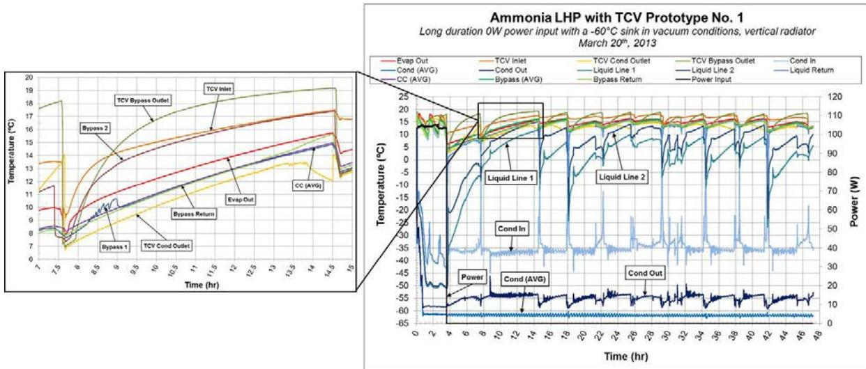
Figure 10. Ammonia LHP with TCV operating with a vertical condenser in the thermal vacuum chamber, -60°C constant sink conditions with long duration 0W power input.
