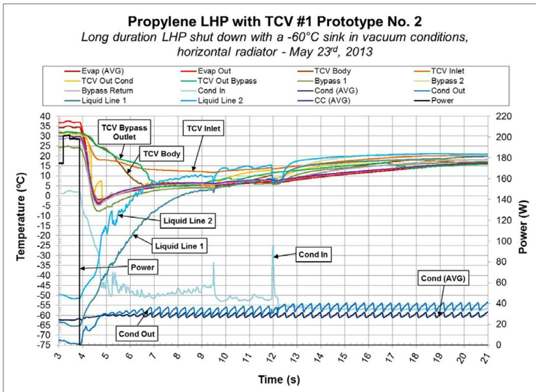
**Figure 16. Propylene LHP with TCV long duration LHP shut down with a  $-60^{\circ}\text{C}$  sink in vacuum conditions with a horizontal condenser.**
