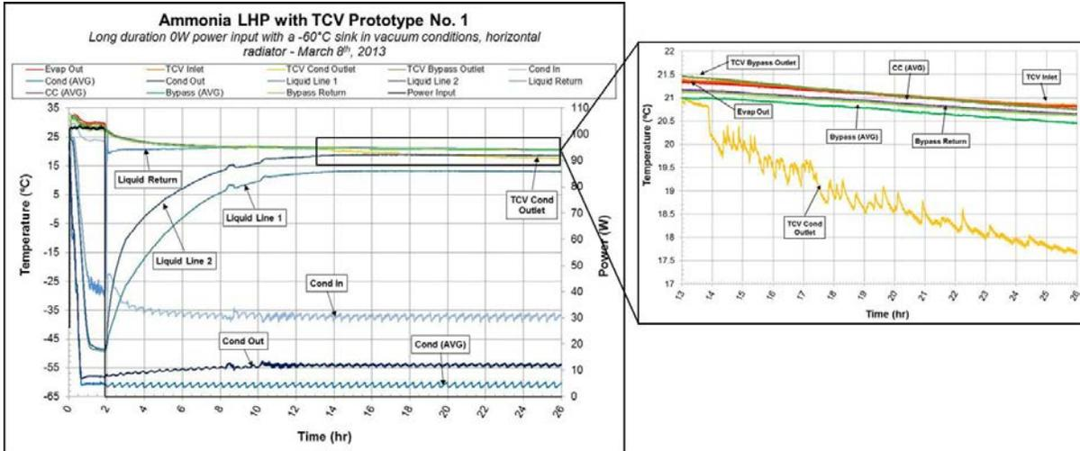
Figure 8. Ammonia LHP with TCV operating with a horizontal condenser in the thermal vacuum chamber, -60°C constant sink conditions with long duration 0W power input.
