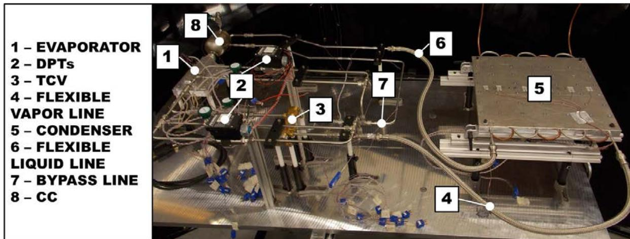
Figure 5. Ammonia LHP with TCV design.
