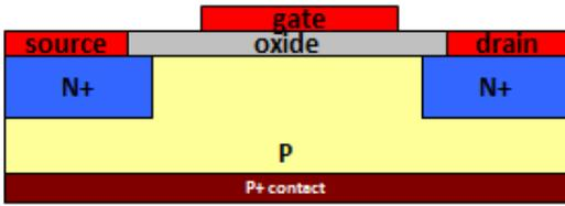
**Figure 3:** A simple SiC MOSFET device for validation ( $1\mu\text{m} \times 0.6\mu\text{m}$ )
