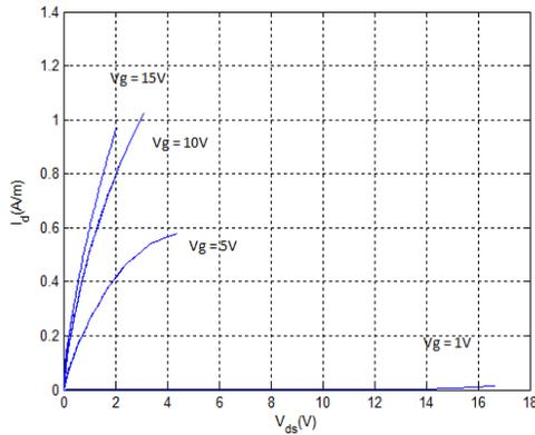
**Figure 6:** Calculated I-V curve under varying gate bias (1V, 5V, 10V, 15V)
