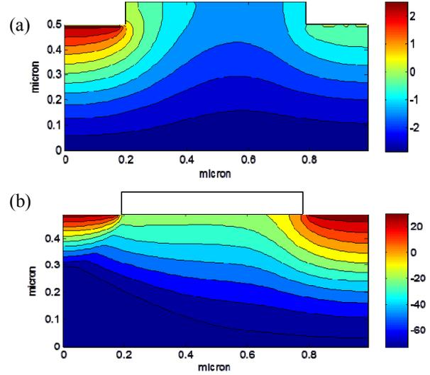
**Figure 4:** OFF-state ( $V_{ds} = 2.6\text{V}$ ,  $V_{gs} = -1\text{V}$ ). (a) Potential V, Volts; (b) electron number density  $n$ ,  $\text{cm}^{-3}$  in log scale
