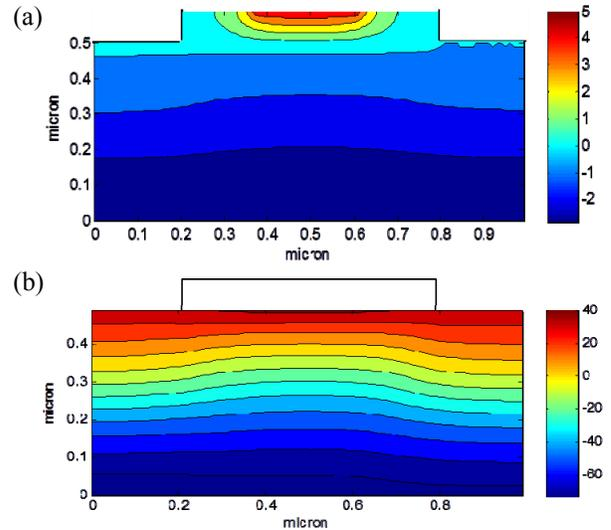
**Figure 5:** ON-state ( $V_{ds} = 0.1\text{V}$ ,  $V_{gs} = 5\text{V}$ ). (a) Potential V, Volts; (b) electron number density  $n$ ,  $\text{cm}^{-3}$  in log scale
