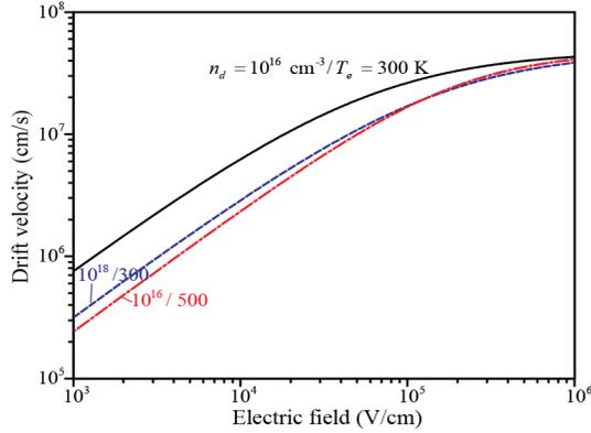
**Figure 2:** Drift velocity in 4H-SiC is a function of electric field, electron number density  $n_d$  and electron temperature  $T_e$ . In the low field region, the drift velocity is proportional to the electric field. In the high field, the drift saturates and becomes independent of the electron number density and electron temperature.
