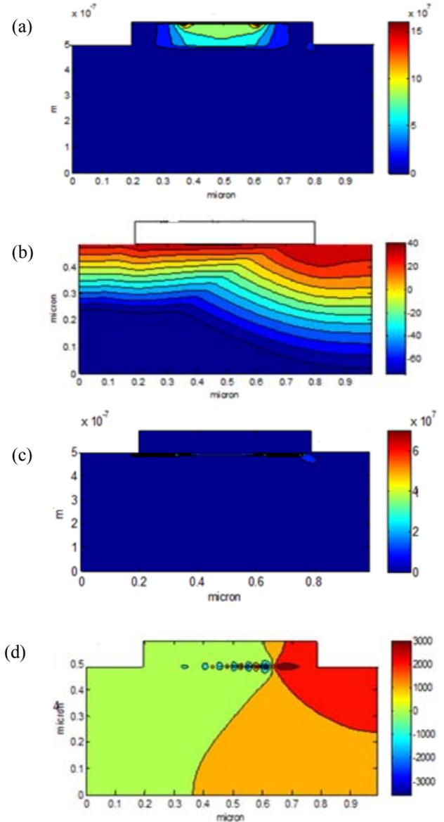
**Figure 7:** Calculated result under  $V_{ds} = 2.2$  V and  $V_{gs} = 10$  V. (a) Electric field  $E$ , V/m; (b) electron number density  $n$ ,  $\text{cm}^{-3}$  in log scale; (c) electron current density  $J$ , A/m<sup>2</sup>; (d) electron temperature  $T_e$ , K.
