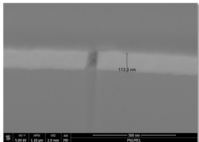
Figure 9. SEM image of coating thickness measurement in microchannel (Point 3 in Figure 6).
