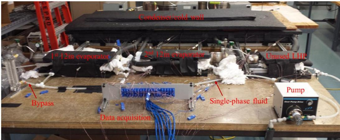
**Figure 8. Photograph of fully assembled and insulated multiple LHP variable heat rejection test setup.**
