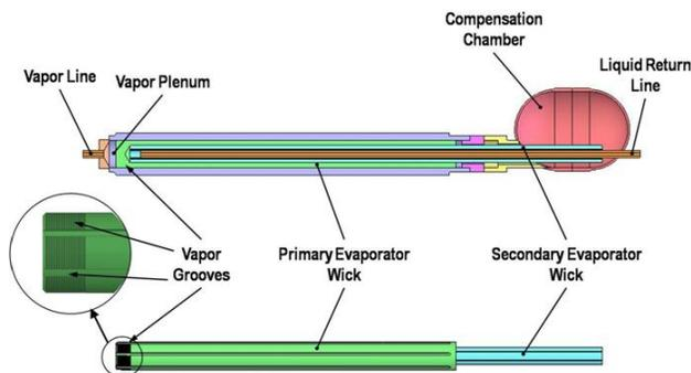
Figure 2. Detailed view of LHP evaporator/compensation chamber assembly
