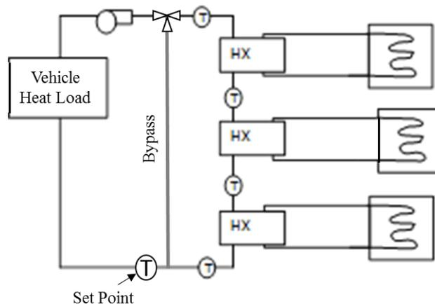
Figure 3. Conceptual multi-LHP system architecture; 3 LHPs are shown
