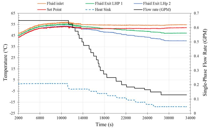
**Figure 11. Water temperature entering and exiting each LHP heat spreader, along with water flow rate. Note how the set point temperature is maintained as the sink temperature and local water flow rate are reduced.**
