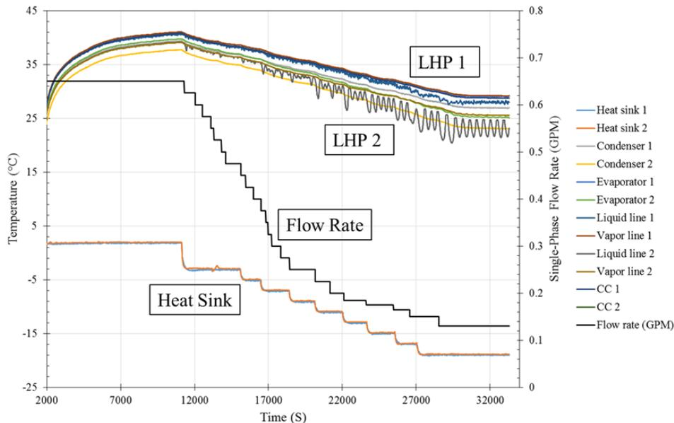
**Figure 9. LHP component temperatures recorded as heat sink temperature is reduced from 2°C to -18°C. Local water flow rate is also shown.**
