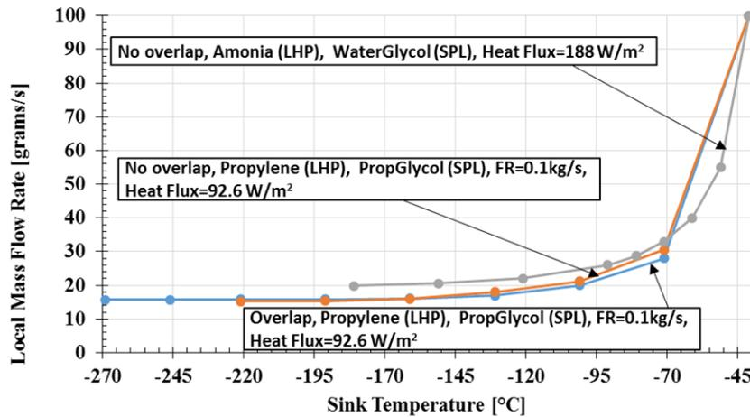
**Figure 4. Local mass flow rate required to maintain set point temperature while sink temperature changes for constant power (2500 W).**
