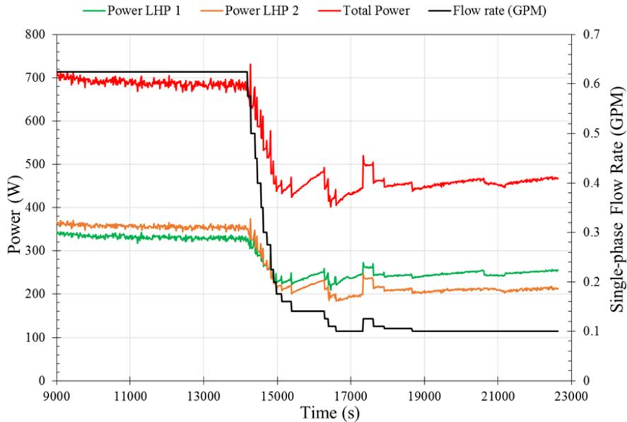
**Figure 14. Heat rejected by each LHP, along with local water flow rate. As the total power applied is reduced, the local water flow rate is reduced to maintain the outlet set point temperature (not shown).**
