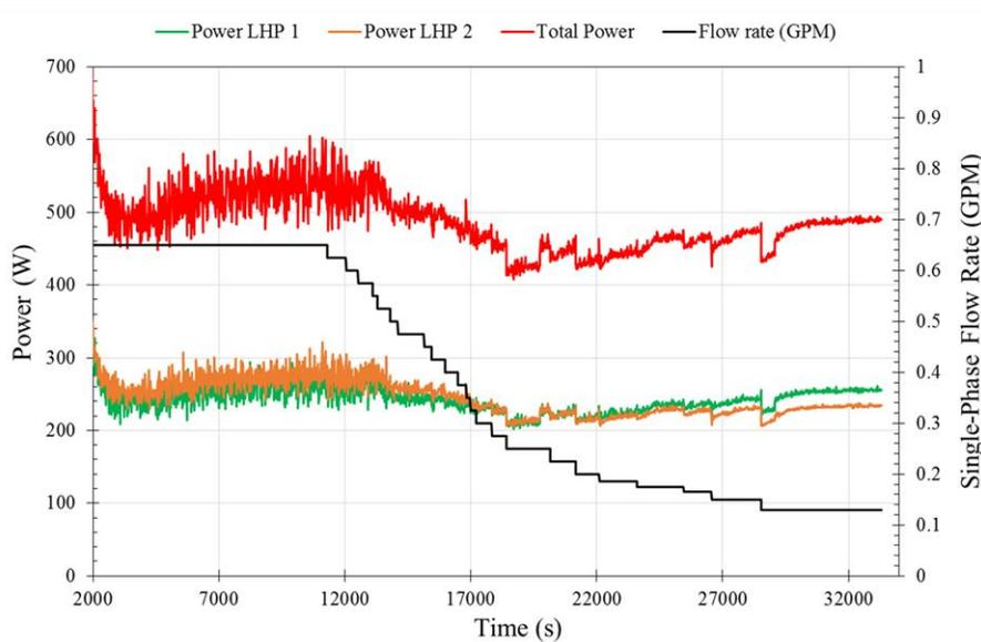
**Figure 10. Heat rejected by each LHP, along with local water flow rate. Note how total rejected power remains fairly constant as the local water flow rate is reduced.**
