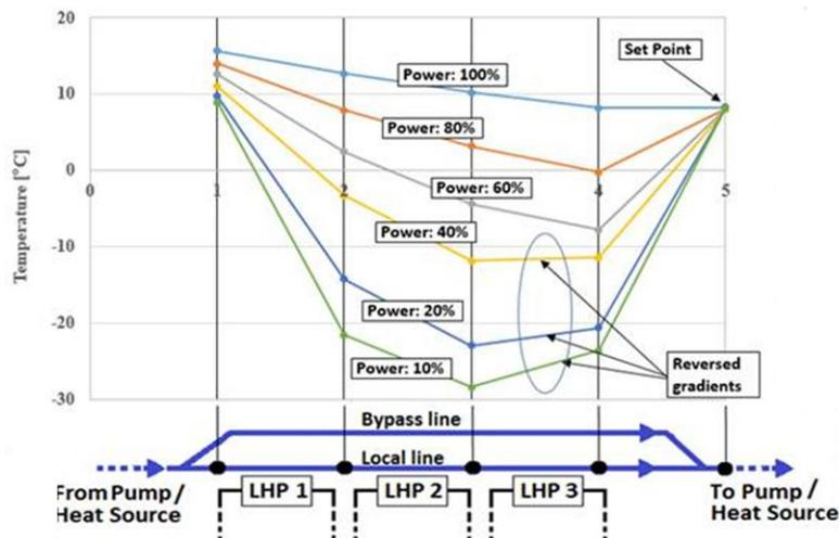
**Figure 7. Temperature distribution along local portion of single-phase loop as power changes for a sink temperature of  $-41^{\circ}\text{C}$ .**
