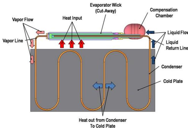
Figure 1. Schematic of a typical LHP (not to scale)
