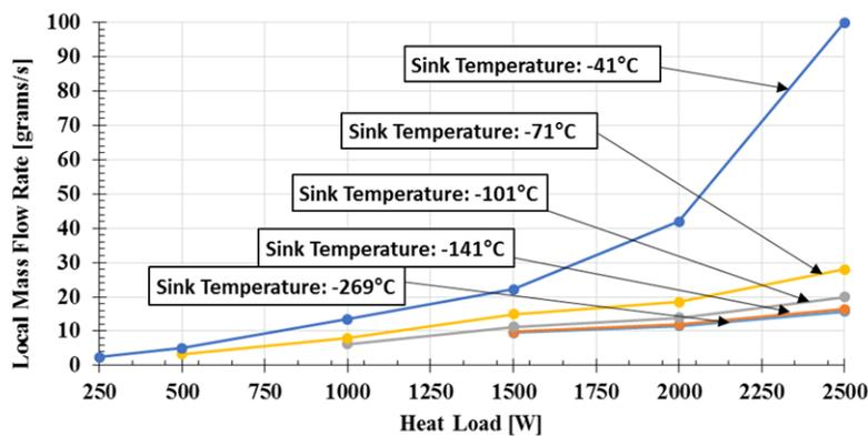
**Figure 5. Local mass flow rate required to maintain set point temperature as heat load changes for constant sink temperature.**
