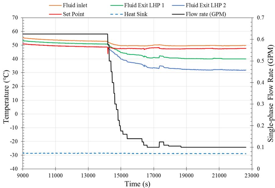
**Figure 13. Water temperature entering and exiting each LHP heat spreader, along with local water flow rate. Note how the temperature of the set point is maintained as the power applied and local water flow rate are reduced.**
