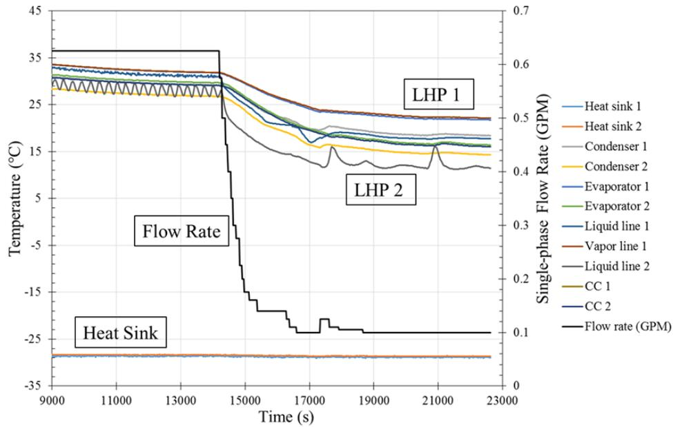
**Figure 12. LHP component temperatures recorded as heat load is reduced for a constant sink temperature. Local water flow rate is also shown.**
