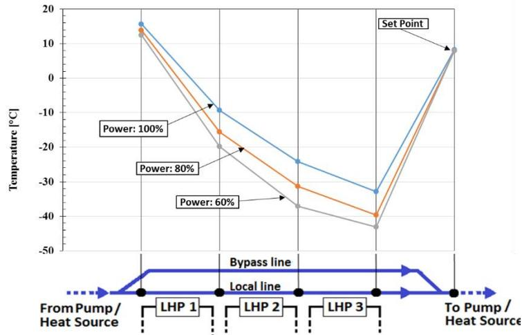
**Figure 6. Temperature distribution along local portion of single-phase loop as power changes for a sink temperature of  $-269^{\circ}\text{C}$ .**
