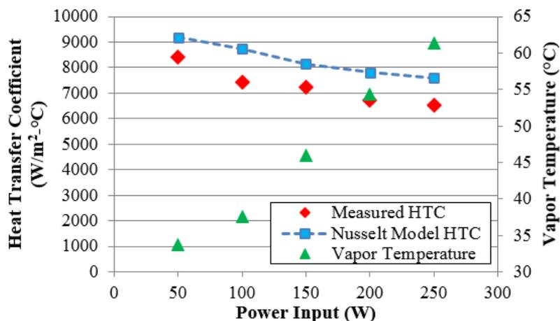
**Fig. 3** Heat transfer coefficients on the plain copper bare surface.
