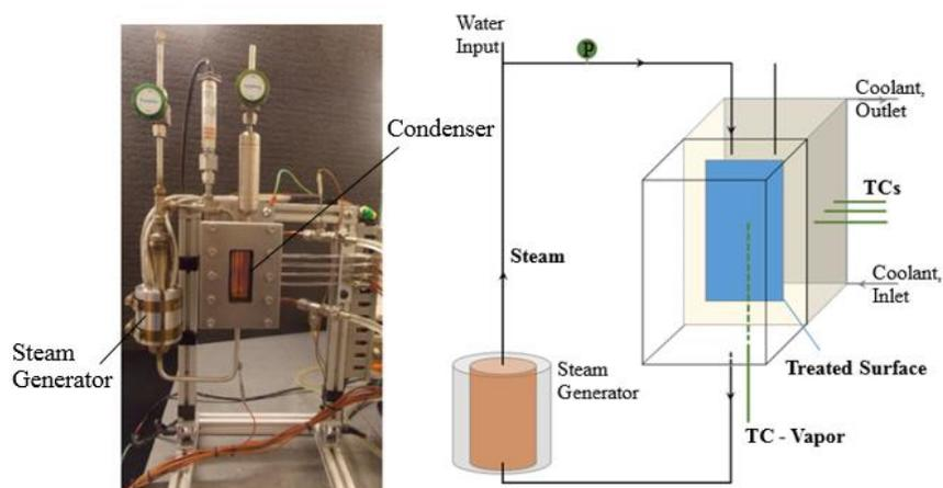
**Fig. 1** Test apparatus for measurement of heat transfer performance on condensing surface.
