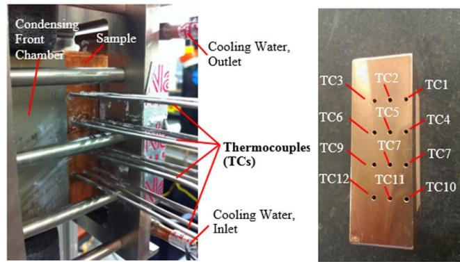
**Fig. 2** Thermocouples arrangements in the test apparatus for determination of heat transfer coefficient on condensation.
