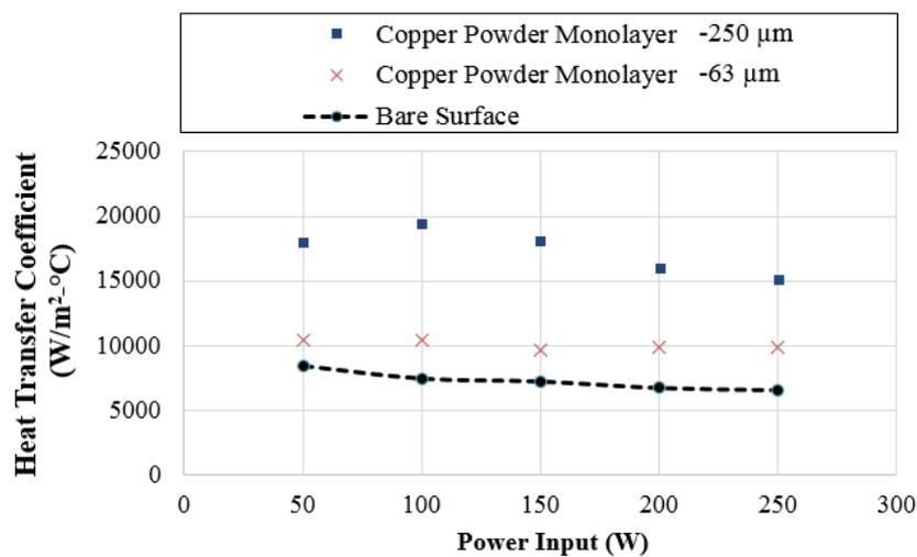
**Fig. 4** Measurements of heat transfer coefficient on hydrophilic surfaces with copper powder.
