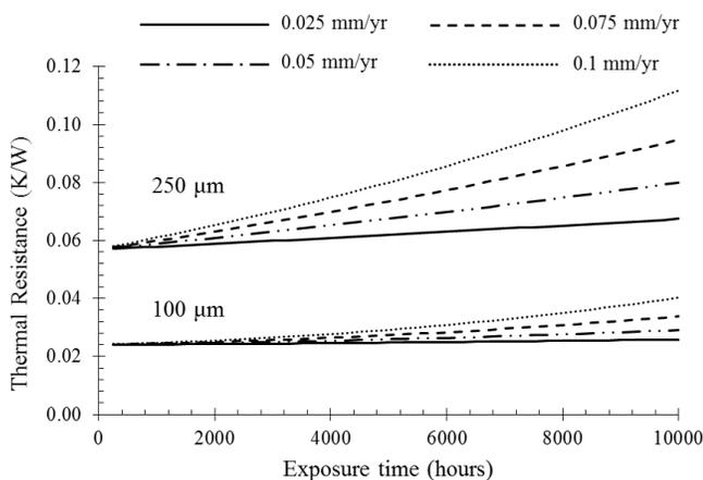
Fig. 16 Change in thermal resistance of a theoretical copper MCC with 100  $\mu\text{m}$  and 250  $\mu\text{m}$  channels, at different constant erosion-corrosion rates
