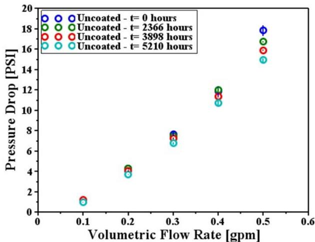
Fig. 6 DIW coolant pressure loss across the baseline uncoated MCC stack over a range of flow rates at several life test time points
