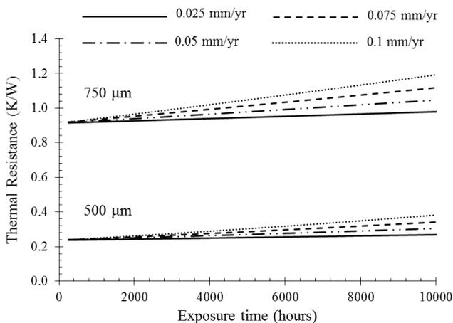
Fig. 17 Change in thermal resistance of a theoretical copper MCC with 500  $\mu\text{m}$  and 750  $\mu\text{m}$  channels, at different constant erosion-corrosion rates
