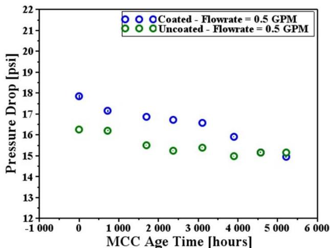
Fig. 8 Evolution of coolant pressure loss over test duration at a flow rate of 0.5 GPM
