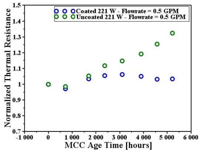
Fig. 14 Evolution of normalized MCC stack thermal resistance over test duration at a flow rate of 0.5 GPM
