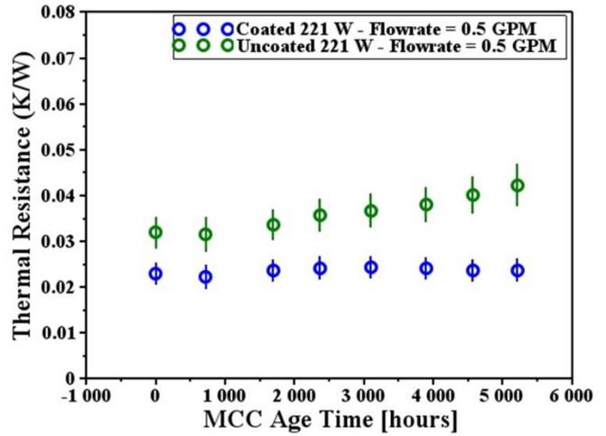
Fig. 12 Evolution of MCC stack thermal resistance of test duration at a flow rate of 0.5 GPM
