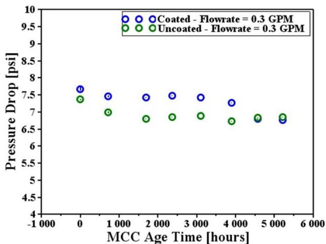
Fig. 7 Evolution of coolant pressure loss over test duration at a flow rate of 0.3 GPM
