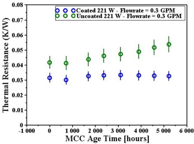
Fig. 11 Evolution of MCC stack thermal resistance over test duration at a flow rate of 0.3 GPM
