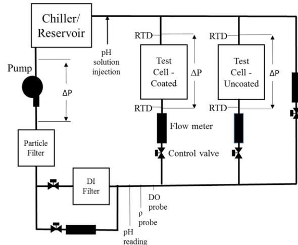
Fig. 2 Schematic of long term MCC life test apparatus [6]
