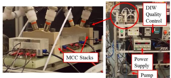
Fig. 3 Long term MCC life test apparatus [6]
