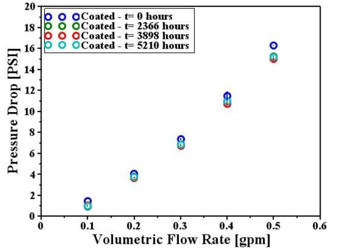
Fig. 5 DIW coolant pressure loss across the coated MCC stack over a range of flow rates at several life test time points
