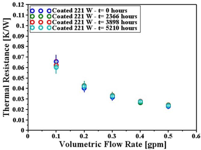
Fig. 9 Total thermal resistance of the coated MCC stack over a range of flow rates at several life test time points
