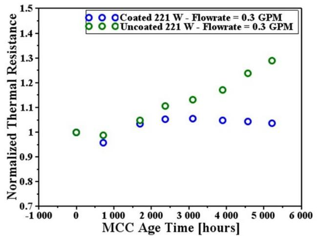
Fig. 13 Evolution of normalized MCC stack thermal resistance over test duration at a flow rate of 0.3 GPM
