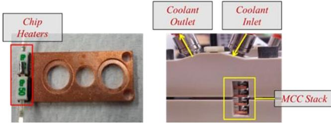
Fig. 4 Resistive heaters soldered to surface of copper MCCs to simulate laser diode waste heat (Left). Four MCCs integrated into a stack for life testing (Right). [6]
