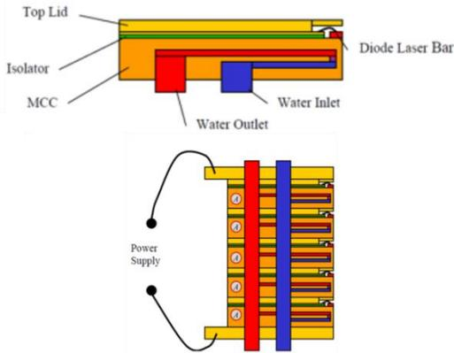
Fig. 1 Copper MCC stack used in laser diode thermal management with parallel cooling paths and series electrical connections [4].
