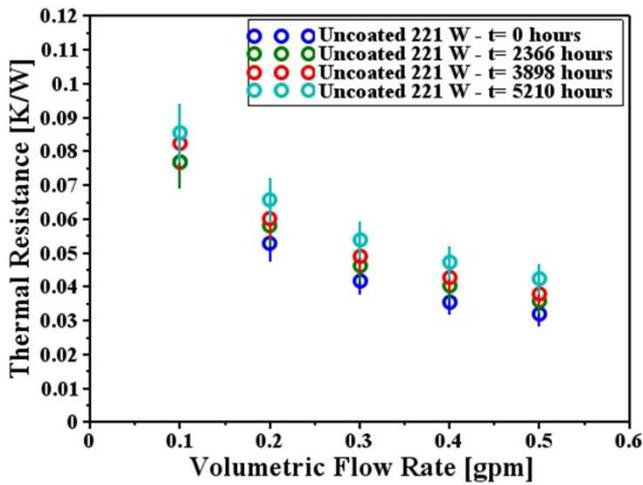
Fig. 10 Total thermal resistance of the baseline uncoated MCC stack over a range of flow rates at several life test time points
