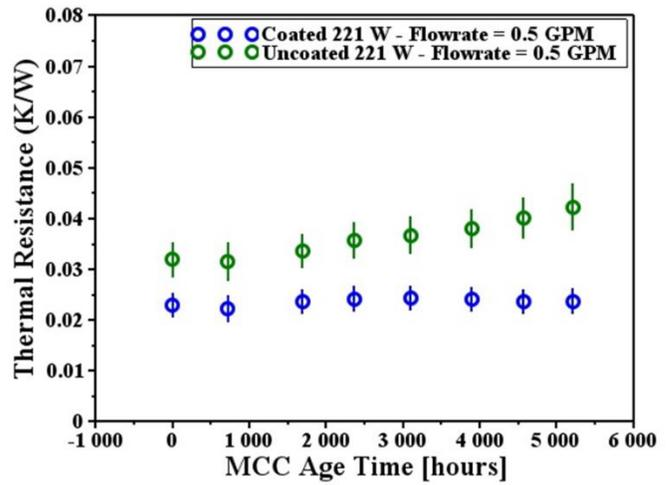
Fig. 12 Evolution of MCC stack thermal resistance of test duration at a flow rate of 0.5 GPM
