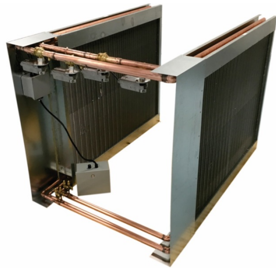
Fig. 4. Split Loop Thermosyphon with Active Control Valves
