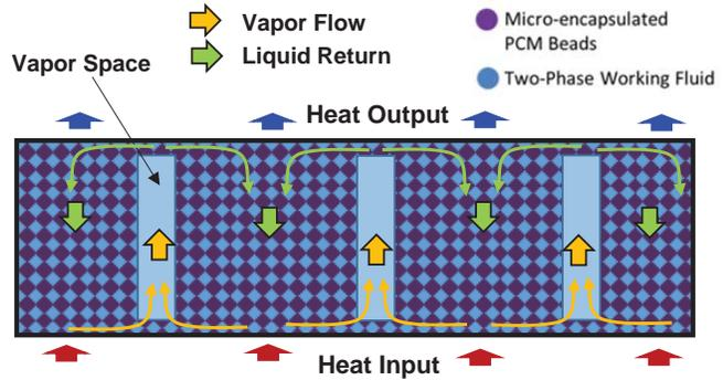
Figure 3. ACT's PCM Vapor Chamber.
