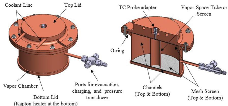
**Figure 5. Copper/Water PCM Vapor Chamber Prototype**
