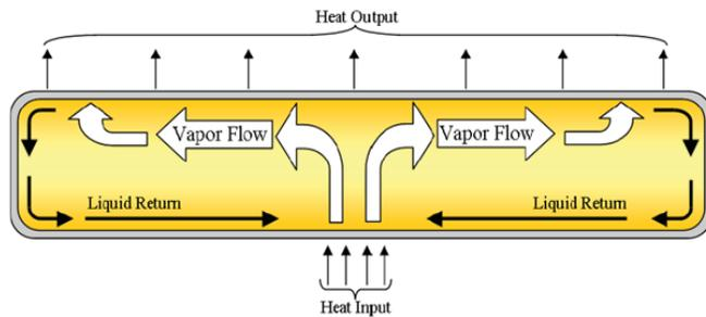
**Figure 2. Standard Vapor Chamber.**
