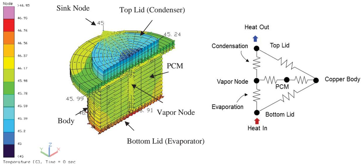
Figure 6. Detailed PCM Vapor Chamber Thermal Model.
