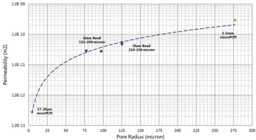
Figure 8. Measured Pore Radius and Permeability.
