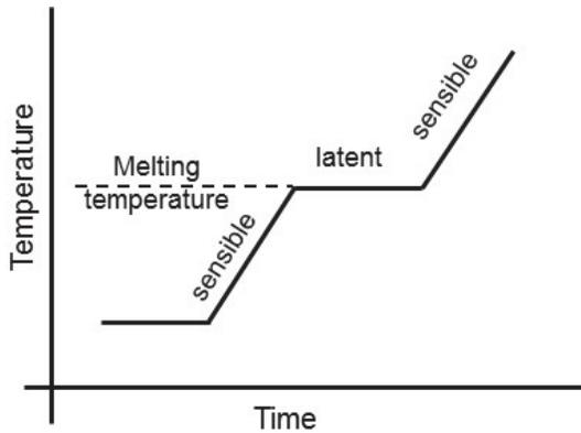
Figure 4. PCM Vapor Chamber Temperature Profile
