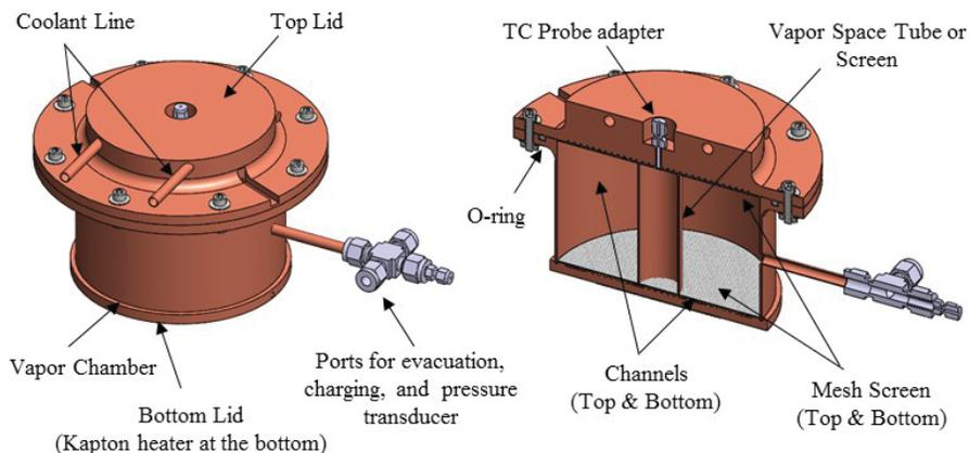
**Figure 5. Copper/Water PCM Vapor Chamber Prototype**
