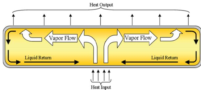
**Figure 2. Standard Vapor Chamber.**
