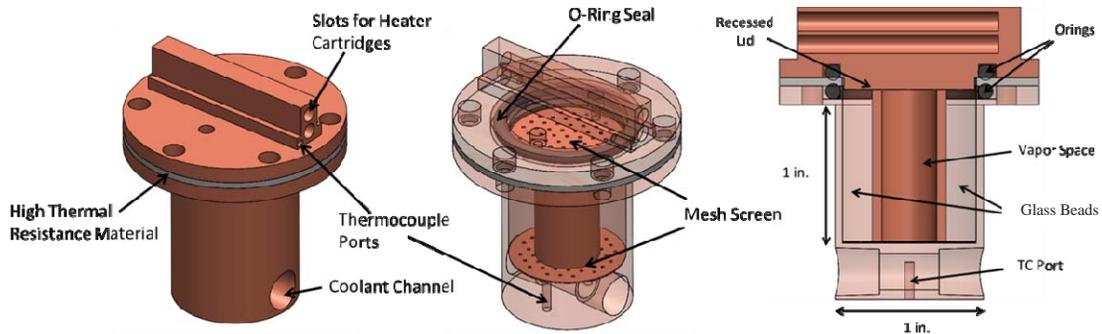
Figure 9. Reduced-scale Proof-of-concept Prototype.
