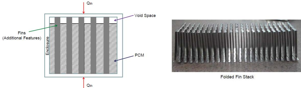
**Figure 1. Folded Fin Stack PCM Heat Sink**
