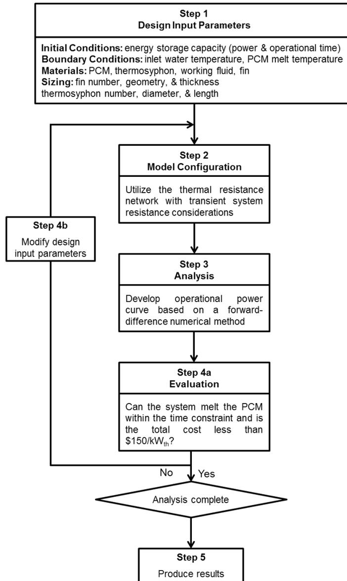
**Fig. 11** Design analysis sequence for the modeling process [8].
