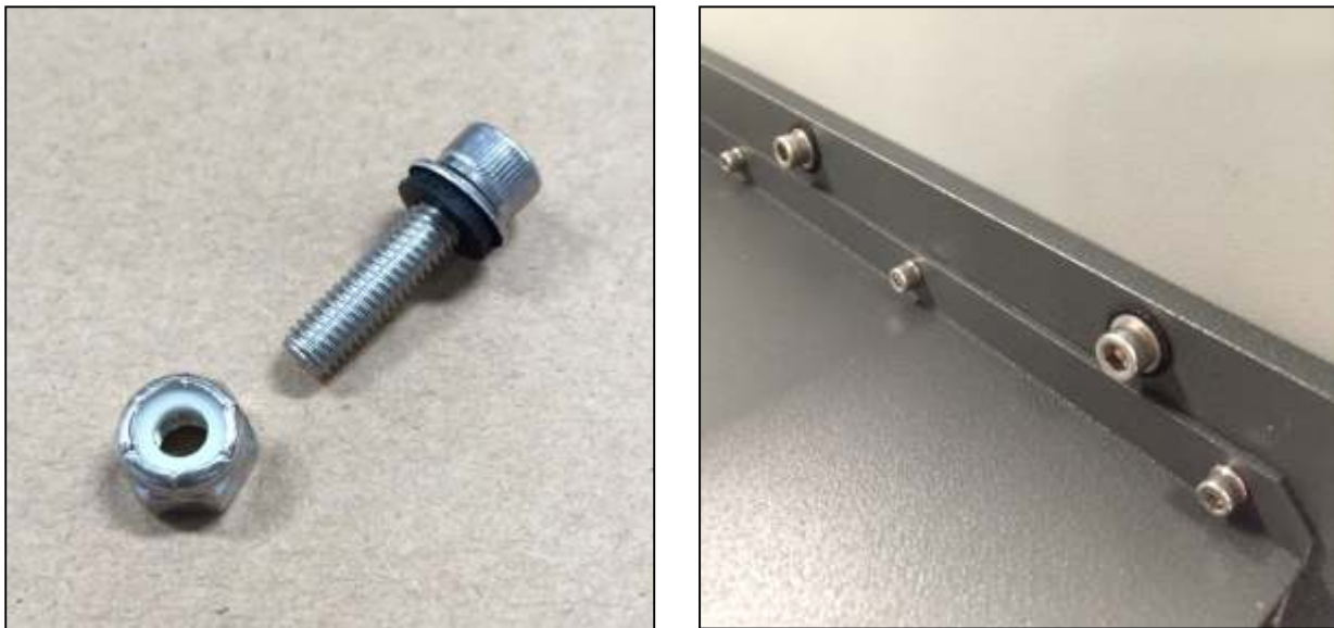
Figure 3: Perimeter bolt with sealing washer and locking nut (left) perimeter bolts installed on enclosure after being torqued down.
