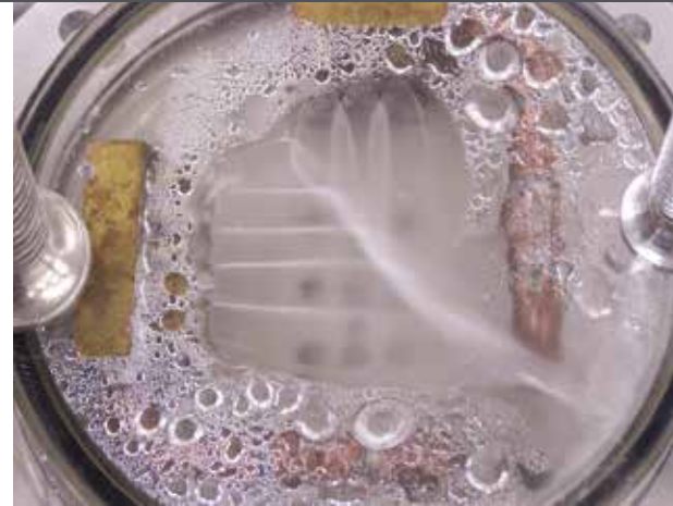
Spray impingement cooling test for prototype high volume optical device development
