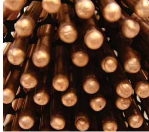
Copper-Water Heat Pipes
