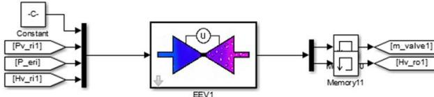
Fig. 3: Electronic Expansion Valve model.
