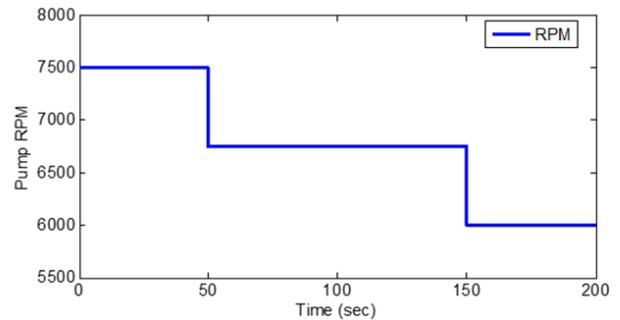
Fig. 15: Pump speed step change.
