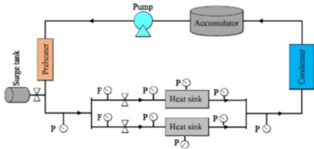
Fig. 12: scaled pumped two-phase system schematic.
