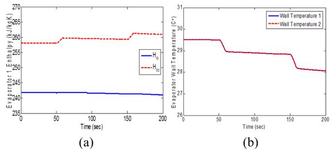
Fig. 17: (a) Evaporator 1 enthalpy response, and (b) Evaporator wall temperature response.
