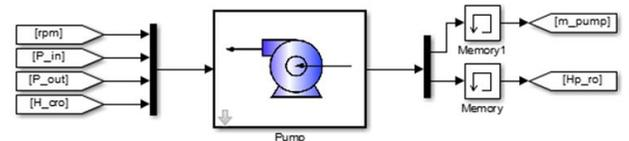
Fig. 2: Semi-empirical variable speed pump model.
