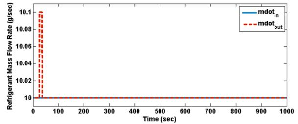
Fig. 9: Refrigerant mass flow rate at evaporator.
