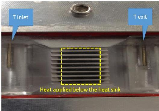
Fig. 14: Mini-channel cold plate.
