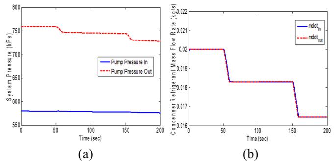
Fig. 16: (a) System pressure response, and (b) Condenser mass flow response.
