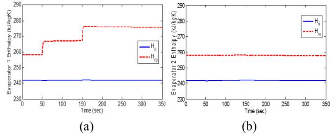
**Fig. 21: Evaporators enthalpy response of (a) Evaporator 1 and (b) Evaporator 2.**
