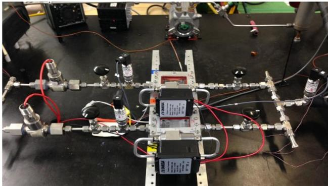
Fig. 13: Pumped two-phase system with two parallel evaporators.
