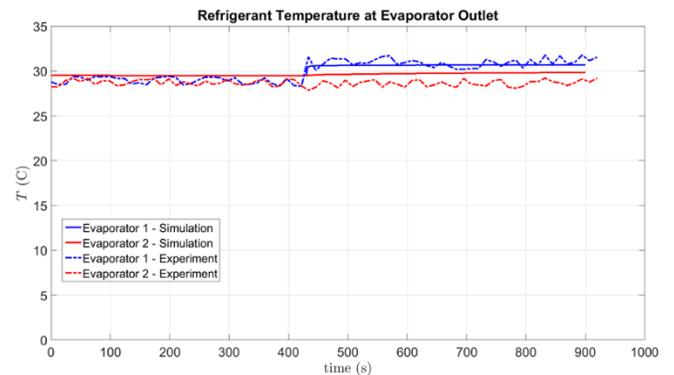
**Fig. 23: Simulation vs Experiment: Refrigerant temperature at evaporator outlet.**
