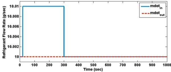
Fig. 6: Refrigerant mass flow rate at evaporator.
