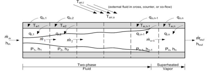
Fig. 1: Finite Control Volume (FCV) heat exchanger model [6].
