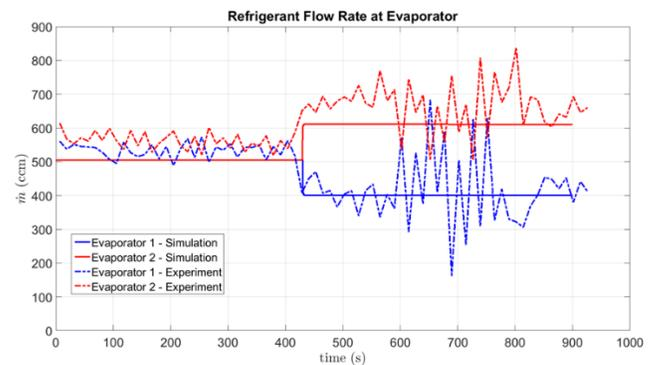
**Fig. 24: Simulation vs Experiment: Refrigerant mass flow rate at each evaporator.**
