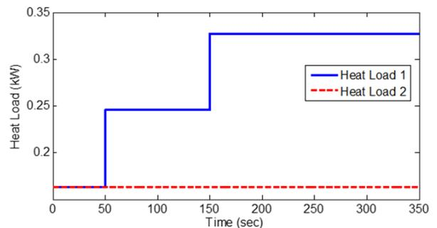
Fig. 18: Step changes in heat load applied to evaporator 1.
