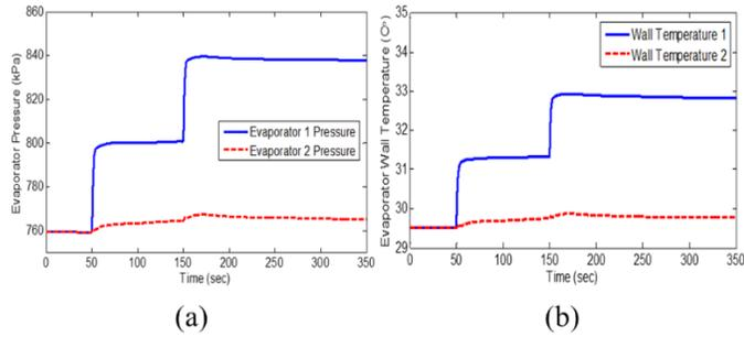
**Fig. 19: (a) Evaporators pressure response and (b) Evaporators wall temperature response.**
