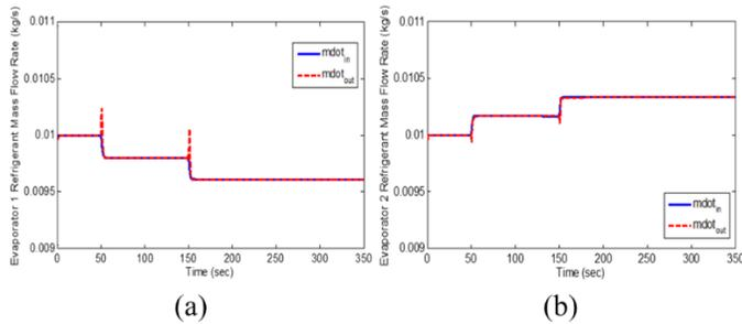
**Fig. 20: Mass Flow Response of (a) Evaporator 1 and (b) Evaporator 2.**
