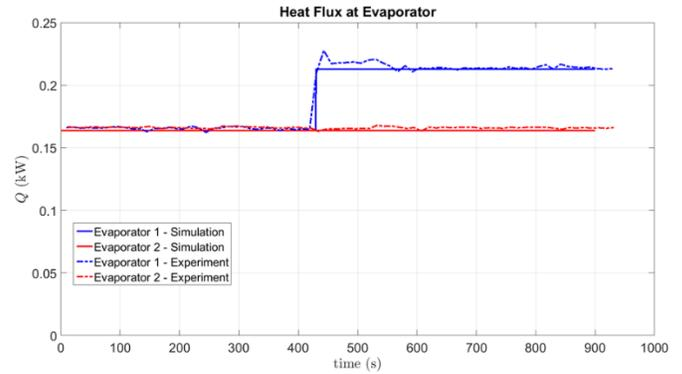
**Fig. 22: Simulation vs Experiment: Step change in heat load.**
