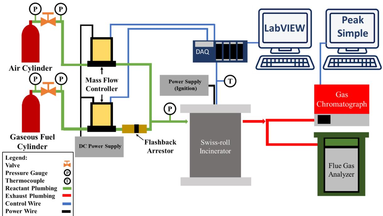
**Figure 6. A schematic of the thermocouple placement during experimental testing of the Swiss-roll incinerator prototype.**
