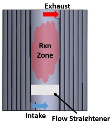
Two cold flow CFD models, with no chemical reaction or heat transfer, were generated by ACT to simulate the performance of the new center design and compare the flow pattern to the standard design. The results in Figure 3, validate the predicted theory as the center velocity vectors in the new design are more uniform in magnitude and direction than the conventional design.
